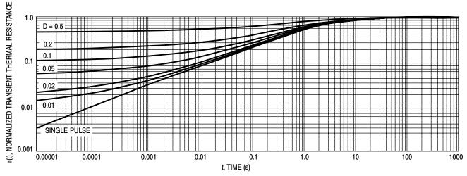
Figure 9. Normalized Thermal Response
