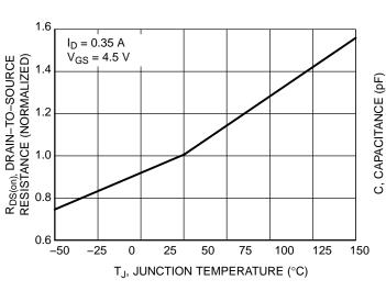
Figure 5. On-Resistance Variation with **Temperature**
