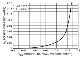
Figure 9. Diode Forward Voltage vs. Current
