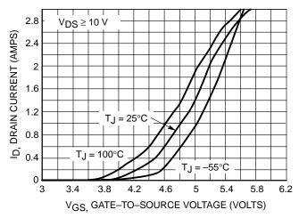
Figure 2. Transfer Characteristics
