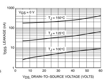
Figure 6. Drain-to-Source Leakage Current versus Voltage
