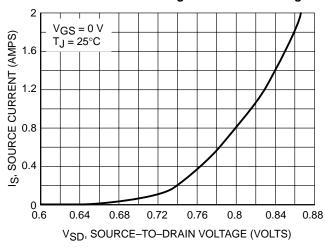
Figure 10. Diode Forward Voltage versus Current
