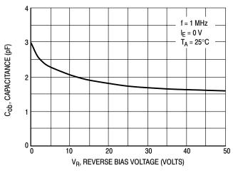
Figure 9. Output Capacitance
