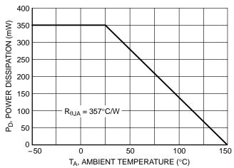
Figure 1. Derating Curve
