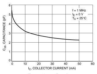
Figure 4. Output Capacitance
