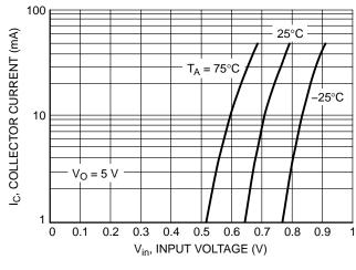
Figure 5. Output Current versus Input Voltage
