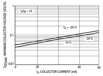
Figure 7.  $V_{CE(sat)}$  versus  $I_C$
