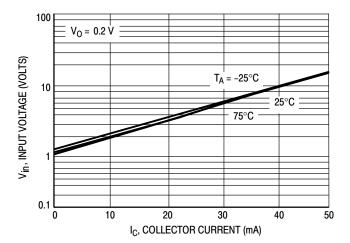
Figure 11. Input Voltage versus Output Current
