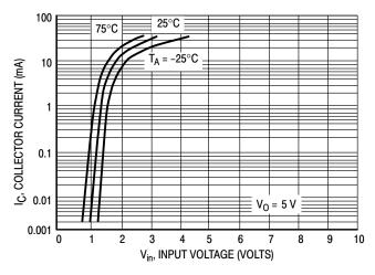
Figure 10. Output Current versus Input Voltage
