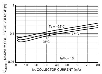
Figure 2. Maximum Collector Voltage versus Collector Current
