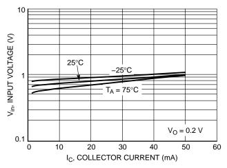
Figure 6. Input Voltage versus Output Current
