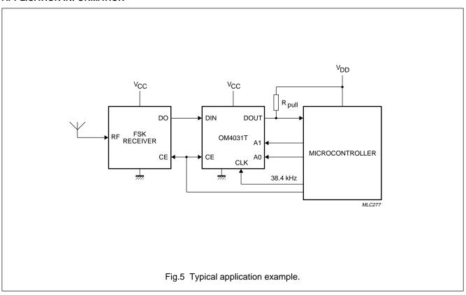
The OM4031T will generally operate from the same power supply ( $V_{CC}$ ) as the FSK data receiver providing its input data. The open-drain data output allows level shifting of the data to suit a microcontroller operating at a higher power supply voltage ( $V_{DD}$ ).
