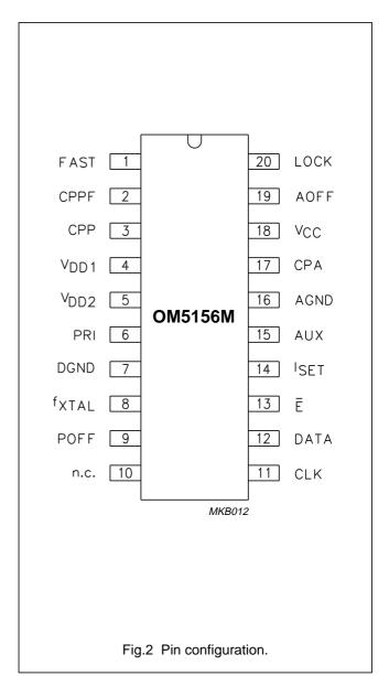
The PRI input (pin 6) drives a preamplifier to provide the clock to the first divider stage. The preamplifier has a high input impedance, dominated by pin and pad capacitance. The circuit operates with signal levels from 60 to 400 mV (RMS), and at frequencies up to 2 GHz. The high frequency divider circuits use bipolar transistors, slower bits are CMOS. Divider ratios (512 to 131071) allow up to 2 MHz phase comparison frequency.
