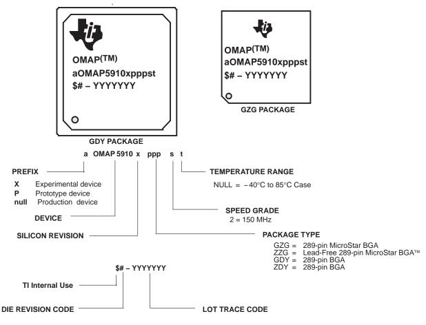
Figure 1. Example Markings for OMAP5910 Packages, Revision J
