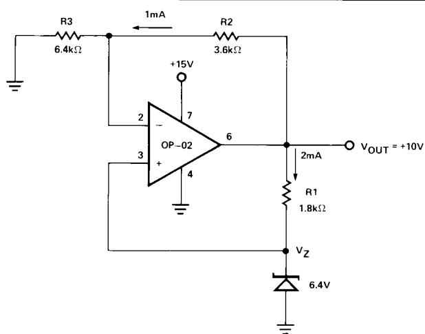
$$V_{OUT} = \left(1 + \frac{R_2}{R_3}\right)V_Z$$
