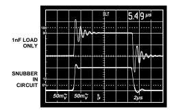
Figure 54. Overshoot and Ringing Is Reduced by Adding a "Snubber" Network in Parallel with the 1 nF Load
