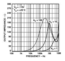
Figure 21. Output Impedance vs. Frequency
