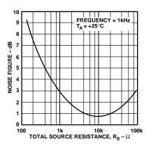
Figure 47. OP284 Noise Figure vs. Source Resistance
