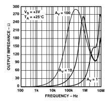
Figure 22. Output Impedance vs. Frequency
