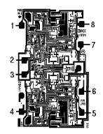
*OP284 Die Size 0.065 × 0.092 Inch, 5,980 Sq. Mils Substrate (Die Backside) Is Connected to V–. Transistor Count, 62.*
