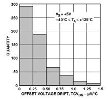
*Figure 5. Input Offset Voltage Drift Distribution*
