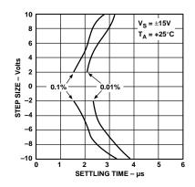
Figure 32. Settling Time vs. Step Size
