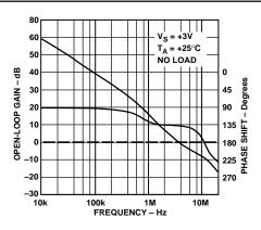
Figure 14. Open-Loop Gain and Phase vs. Frequency (No Load)
