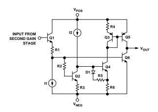
Figure 42. OP284 Equivalent Output Circuit
