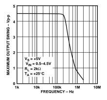
Figure 23. Maximum Output Swing vs. Frequency
