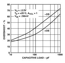
Figure 27. Small Signal Overshoot vs. Capacitive Load
