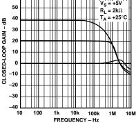
Figure 17. Closed-Loop Gain vs. Frequency (2  $k\Omega$  Load)
