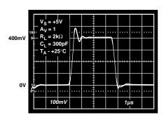
Figure 37. Small Signal Transient Response
