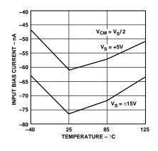
Figure 7. Bias Current vs. Temperature
