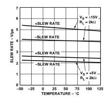
Figure 28. Slew Rate vs. Temperature
