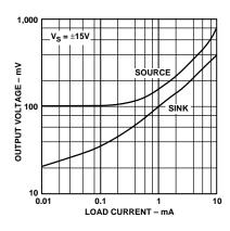
Figure 9. Output Voltage to Supply Rail vs. Load Current
