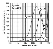
Figure 20. Output Impedance vs. Frequency
