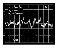
Figure 34. 0.1 Hz to 10 Hz Noise
