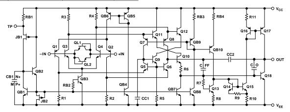
Figure 1. Simplified Schematic
