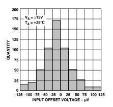
Figure 4. Input Offset Voltage Distribution
