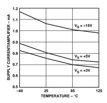
*Figure 10. Supply Current vs. Temperature*
