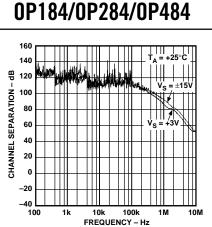
Figure 35. Channel Separation vs. Frequency
