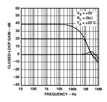
Figure 19. Closed-Loop Gain vs. Frequency (2  $k\Omega$  Load)
