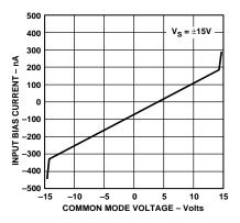
Figure 8. Input Bias Current vs. Common-Mode Voltage
