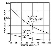
Figure 16. Open-Loop Gain vs. Temperature
