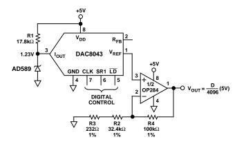
Figure 51. A +5 V Only, 12-Bit DAC Swings Rail-to-Rail
