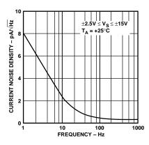
Figure 30. Current Noise Density vs. Frequency
