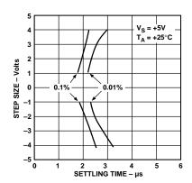
Figure 31. Settling Time vs. Step Size
