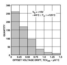
Figure 6. Input Offset Voltage Drift Distribution
