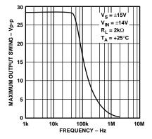
Figure 24. Maximum Output Swing vs. Frequency
