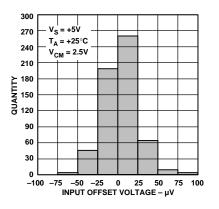
*Figure 3. Input Offset Voltage Distribution*
