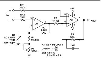
Figure 49. A Single Supply, +3 V Low Noise Instrumentation Amplifier
