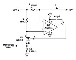
Figure 52. A High-Side Load Current Monitor
