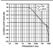
TPC 10. Closed-Loop Gain vs. Frequency,  $V_S = 3 V$
