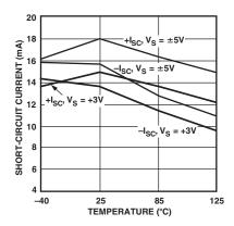
TPC 34. Short-Circuit Current vs. Temperature,  $V_S = +3 V$ ,  $\pm 5 V$
