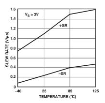
TPC 15. Slew Rate vs. Temperature,  $V_S = 3 V$
