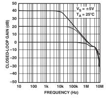
TPC 45. Closed-Loop Gain vs. Frequency,  $V_S = \pm 5 \text{ V}$
