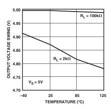
TPC 25. Output Voltage Swing vs. Temperature,  $V_S = 5 \text{ V}$
