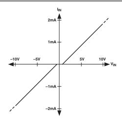
Figure 3. Input Overvoltage Characteristics
