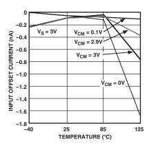
TPC 5. Input Offset Current vs. Temperature,  $V_S = 3 V$
