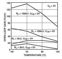
TPC 27. Open-Loop Gain vs. Temperature,  $V_S = 5 V$
