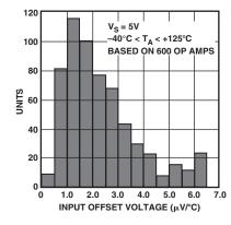
TPC 20. OP291 Input Offset Voltage Drift Distribution,  $V_S = 5 V$
