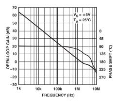
TPC 43. Open-Loop Gain and Phase vs. Frequency,  $V_S = \pm 5 \text{ V}$
