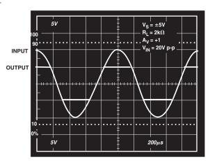
Figure 1. Input and Output with Inputs Overdriven by 5 V
