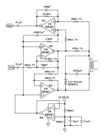
Figure 12. Single-Supply Direct Access Arrangement for Modems
