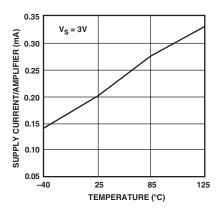
TPC 16. Supply Current vs. Temperature,  $V_S = +3 V$ ,  $\pm 5 V$
