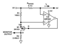
Figure 10. A High-Side Load Current Monitor
