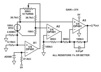
Figure 7. Single-Supply RTD Amplifier
