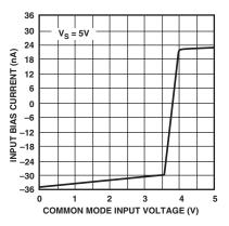
TPC 24. Input Bias Current vs. Common-Mode Input Voltage,  $V_S = 5 V$
