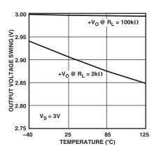
TPC 7. Output Voltage Swing vs. Temperature,  $V_S = 3 V$
