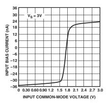
TPC 6. Input Bias Current vs. Input Common-Mode Voltage,  $V_S = 3 V$
