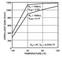
TPC 9. Open-Loop Gain vs. Temperature,  $V_S = 3 V$
