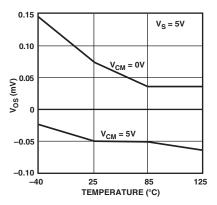
TPC 21. Input Offset Voltage vs. Temperature,  $V_S = 5 V$
