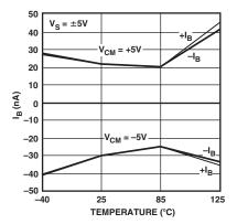
TPC 39. Input Bias Current vs. Temperature,  $V_S = \pm 5 \text{ V}$
