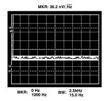
TPC 18. Voltage Noise Density,  $V_S = +3 \text{ V}$  to  $\pm 5 \text{ V}$ ,  $A_{VO} = 1000$
