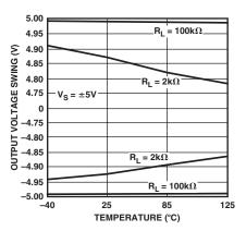
TPC 42. Output Voltage Swing vs. Temperature,  $V_S = \pm 5 V$
