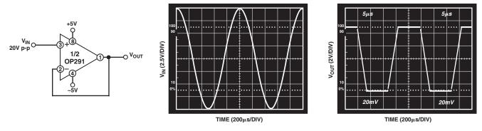
Figure 4. Output Voltage Phase Reversal Behavior
