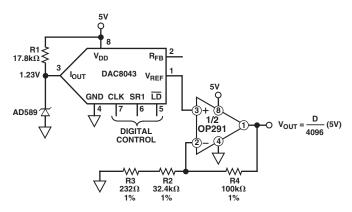
Figure 9. 5 V Only, 12-Bit DAC Swings Rail-to-Rail
