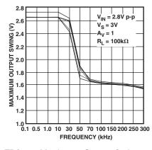
TPC 17. Maximum Output Swing vs. Frequency,  $V_S = 3 V$
