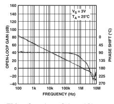
TPC 8. Open-Loop Gain and Phase vs. Frequency,  $V_S = 3 \text{ V}$
