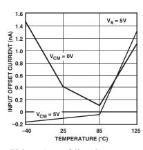
TPC 23. Input Offset Current vs. Temperature,  $V_S = 5 V$
