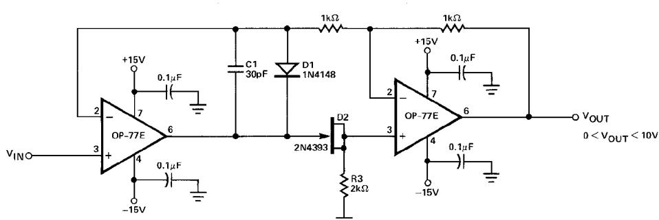
The high gain and low  $TCV_{OS}$  assure accurate operation with inputs from microvolts to volts. In this circuit, the signal always appears as a common-mode signal to
