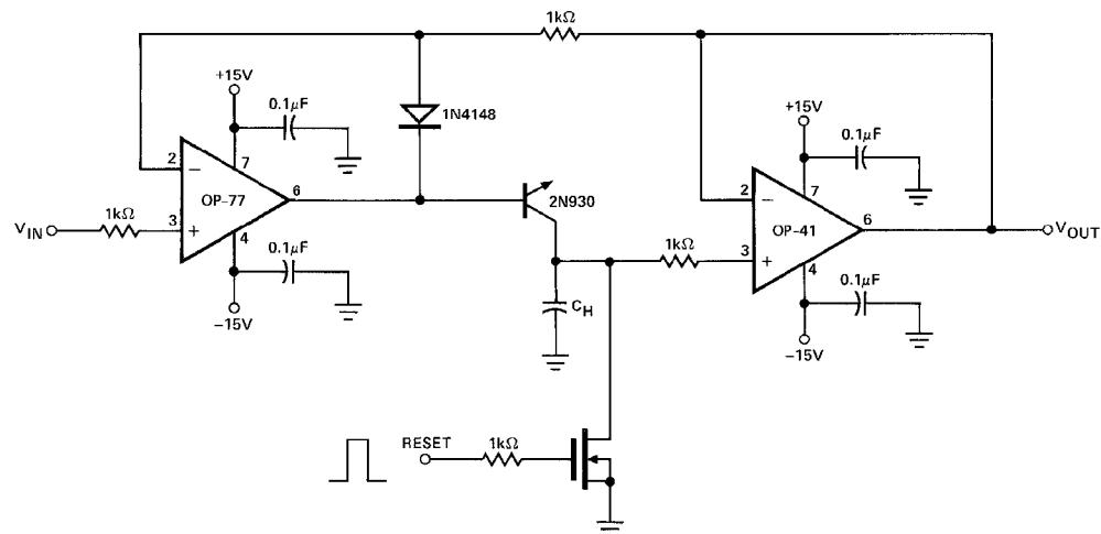
$C_H$  must be of polystyrene, Teflon\*, or polyethylene to minimize dielectric absorption and leakage. The droop
