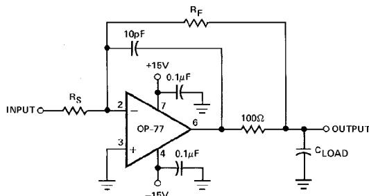
This circuit reduces maximum slew-rate but allows driving capacitive loads of any size without instability. Because the 100Ω resistor is inside the feedback loop, its effect on output impedance is reduced to insignificance by the high open-loop gain of the OP-77.
