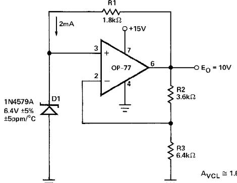
This simple bootstrapped voltage reference provides a precise 10 volts virtually independent of changes in power supply voltage, ambient temperature, and output loading. Correct zener operating current of exactly 2mA is maintained by R1, a selected 5ppm/°C resistor, connected to the regulated output. Accuracy is primarily determined by three factors: the 5ppm/°C temperature coefficient of D1, 1ppm/°C ratio tracking of R2 and R3, and operational amplifier  $V_{OS}$  errors.
