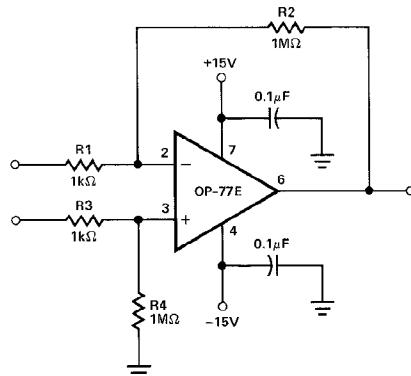
The high gain, gain linearity, CMRR, and low  $TCV_{OS}$  of the OP-77 make it possible to obtain performance not previously available in single stage very high-gain amplifier applications.
