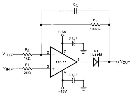
When  $V_{IN} < V_{TH}$ , amplifier output swings negative, reverse biasing diode D1.  $V_{OUT} = V_{TH}$  if  $R_L = \infty$ . When  $V_{IN} \geq V_{TH}$ , the loop closes,
