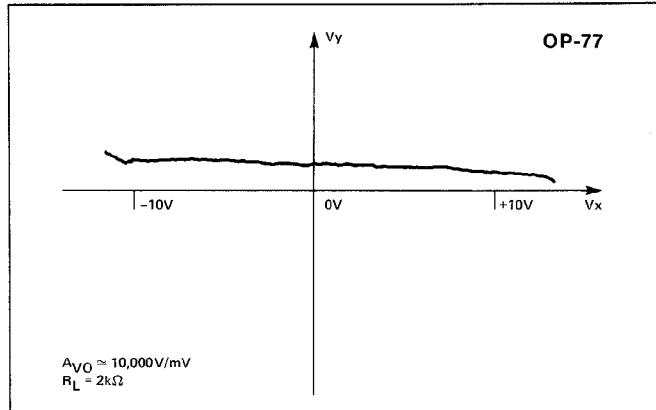
Actual open-loop voltage gain can vary greatly at various output voltages. All automated testers use end-point testing and therefore only show the average gain. This causes errors in high closed-loop gain circuits. Since this is so difficult for manufacturers to test, you should make your own evaluation. This simple test circuit makes it easy. An ideal op amp would show a horizontal scope trace.
