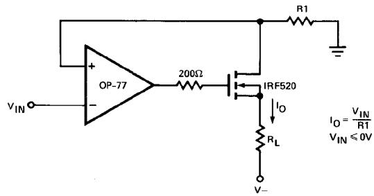
These simple high current sinks require that the load float between the power supply and the sink.
