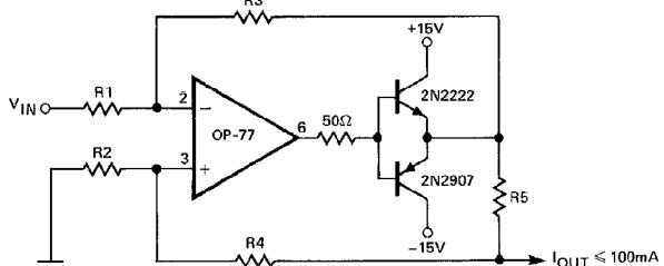
$$I_{OUT} = V_{IN} \frac{R_3}{R_1 \cdot R_5}$$
