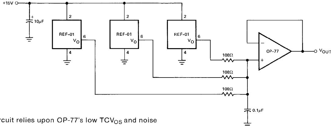
This circuit relies upon OP-77's low  $TCV_{OS}$  and noise combined with very high CMRR to provide precision buffering of the averaged REF-01 voltage outputs.
