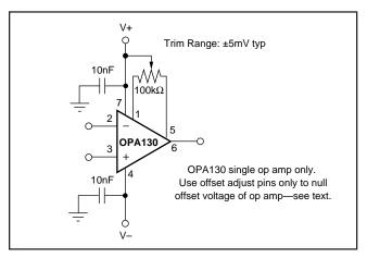
FIGURE 1. OPA130 Offset Voltage Trim Circuit.
