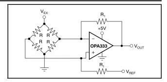
Figure 21. Single Op Amp Bridge Amplifier
