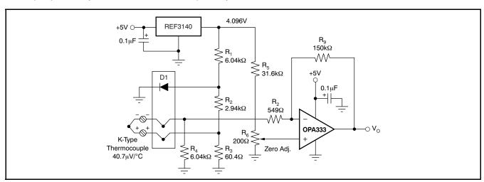
Figure 20. Temperature Measurement
