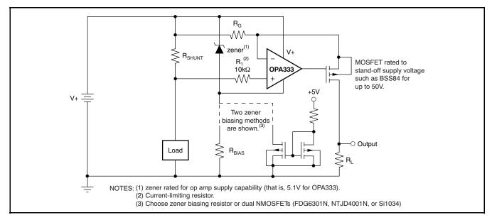
Figure 23. High-Side Current Monitor
