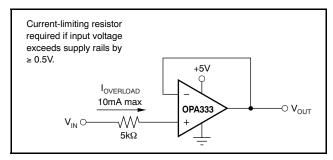
Figure 18. Input Current Protection
