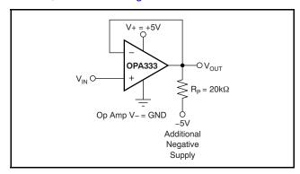
Figure 19. For V<sub>OUT</sub> Range to Ground
