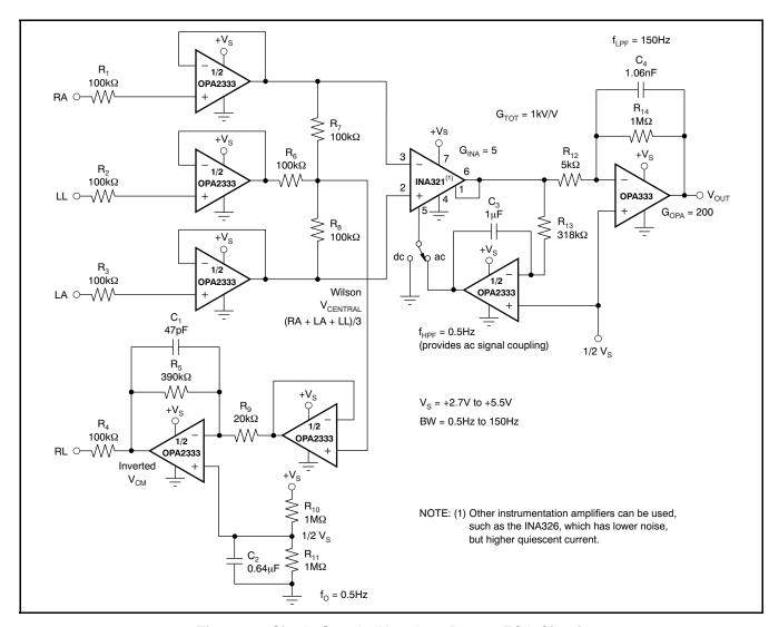
Figure 26. Single-Supply, Very Low Power, ECG Circuit
