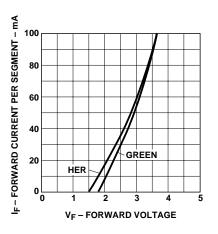
Figure 2. Forward Current vs. Forward Voltage.
