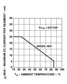
Figure 1. Maximum Allowable DC Current vs. Ambient Temperature.
