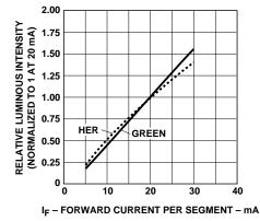
Figure 3. Relative Luminous Intensity vs. DC Forward Current.
