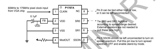
Note: To set the P1707A to standby mode, disable the input clock (pin 1 CLKIN) and pull SSON (pin 5) low. Refer Standby Mode Selection Table.
