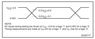
Figure 47. AC Testing Input/Output
