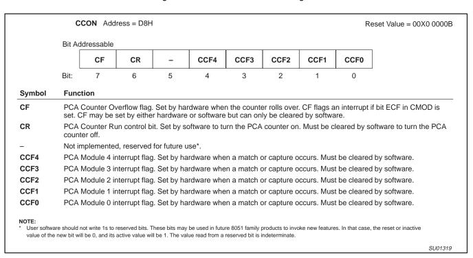
Figure 29. CCON: PCA Counter Control Register
