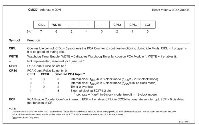
Figure 28. CMOD: PCA Counter Mode Register
