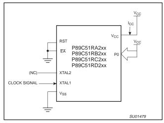
Figure 53.  $I_{CC}$  Test Condition, Idle Mode,  $T_{amb}$  = 25 °C. All other pins are disconnected
