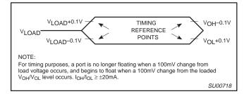
Figure 48. Float Waveform
