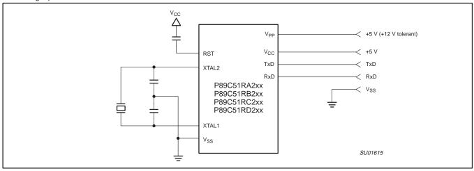
Figure 41. In-System Programming with a Minimum of Pins
