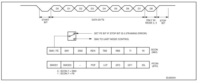
Figure 19. UART Framing Error Detection
