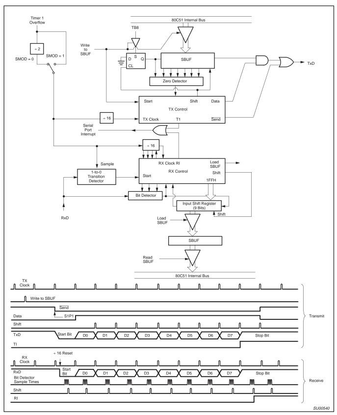
Figure 15. Serial Port Mode 1
