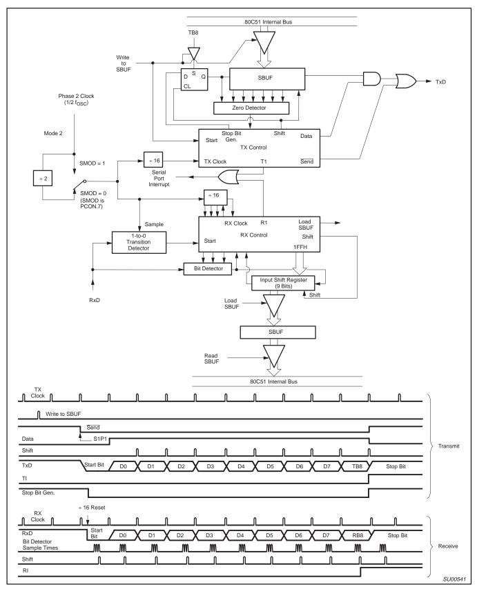
Figure 16. Serial Port Mode 2
