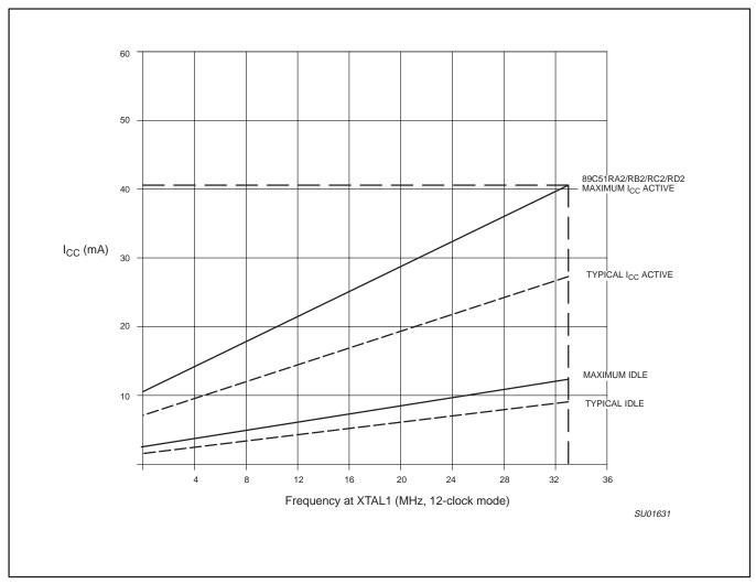
Figure 49. I<sub>CC</sub> vs. FREQ Valid only within frequency specifications of the device under test
