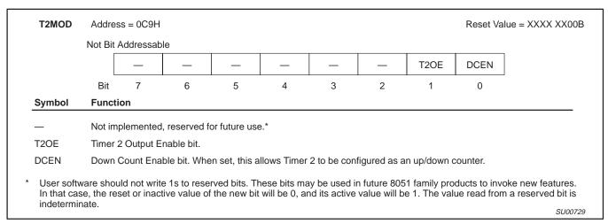
Figure 8. Timer 2 Mode (T2MOD) Control Register
