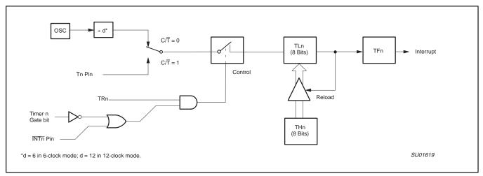
Figure 4. Timer/Counter 0/1 Mode 2: 8-Bit Auto-Reload
