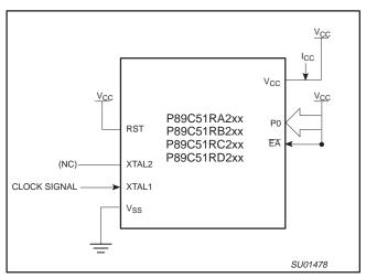
Figure 52.  $I_{CC}$  Test Condition, Active Mode,  $T_{amb}$  = 25 °C. All other pins are disconnected
