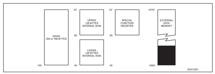
Figure 39. Internal and External Data Memory Address Space with EXTRAM = 0
