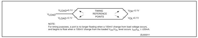
Figure 51. Float Waveform
