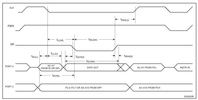
Figure 44. External Data Memory Write Cycle
