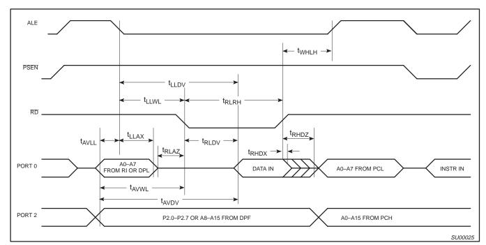
Figure 43. External Data Memory Read Cycle
