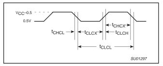
Figure 54. Clock Signal Waveform for  $I_{\mbox{\footnotesize CC}}$  Tests in Active and Idle Modes.
