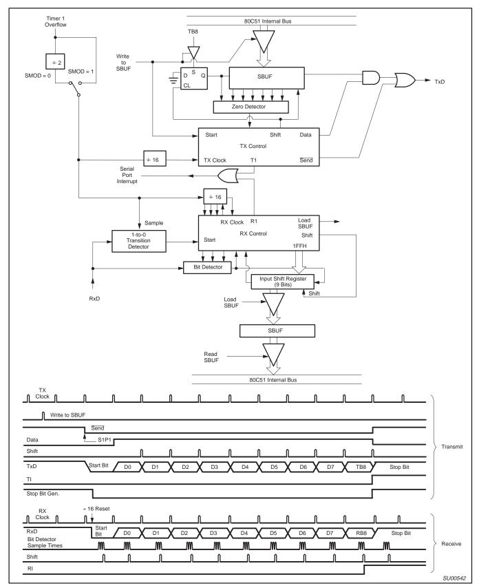
Figure 17. Serial Port Mode 3
