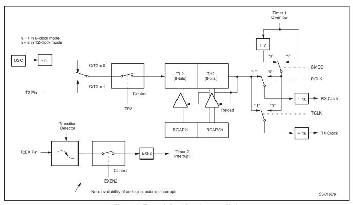
Figure 11. Timer 2 in Baud Rate Generator Mode
