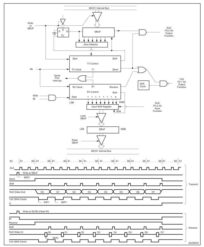
Figure 14. Serial Port Mode 0
