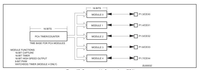
Figure 25. Programmable Counter Array (PCA)
