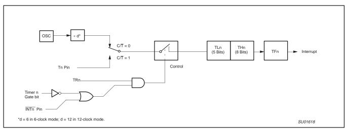
Figure 2. Timer/Counter 0/1 Mode 0: 13-Bit Timer/Counter
