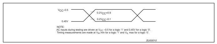
Figure 50. AC Testing Input/Output
