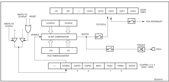
Figure 34. PCA High Speed Output Mode
