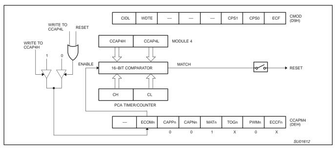
Figure 36. PCA Watchdog Timer mode (Module 4 only)
