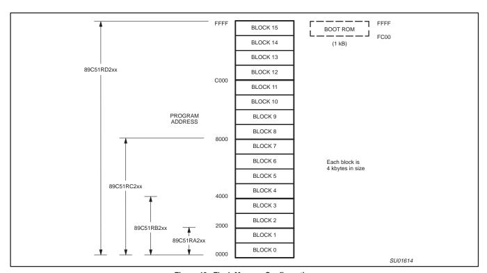
Figure 40. Flash Memory Configurations
