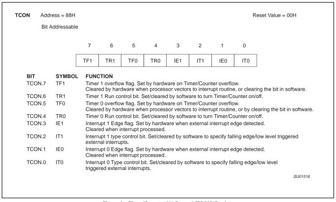
Figure 3. Timer/Counter 0/1 Control (TCON) Register
