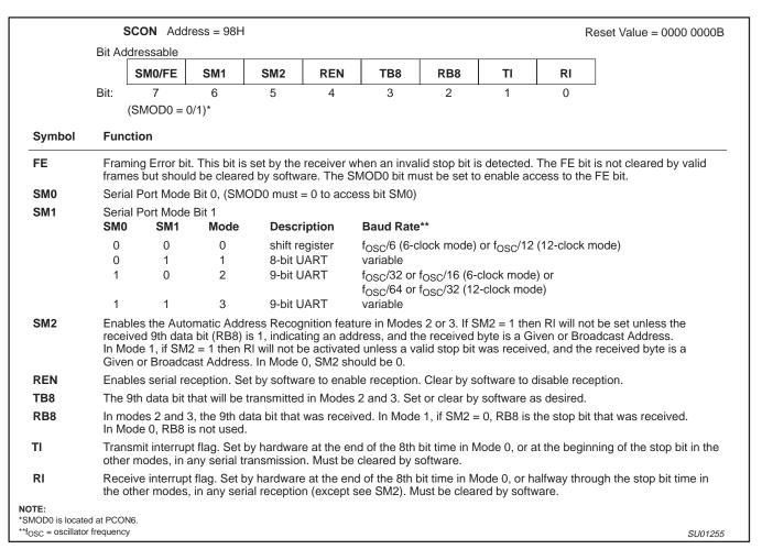
Figure 18. SCON: Serial Port Control Register
