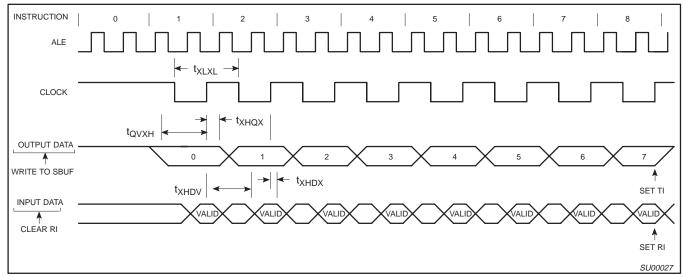
Figure 45. Shift Register Mode Timing
