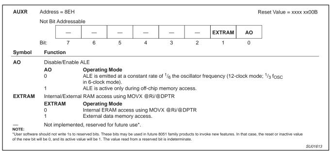
Figure 38. AUXR: Auxiliary Register
