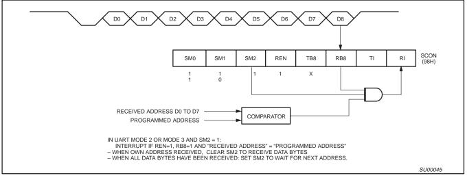
Figure 20. UART Multiprocessor Communication, Automatic Address Recognition
