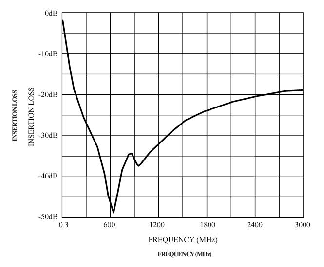
Filter insertion loss is measured using Hewlett Packard HP8753C.
