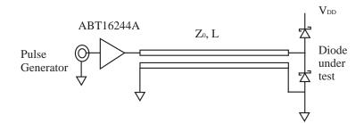
Test Circuit. Line length, pulse width and duty cycle are selected such as that only one reflection is involved in the measurement.
