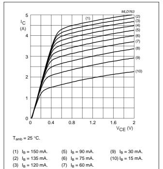
Collector current as a function of collector-emitter voltage; typical values.
