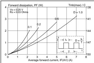
Fig.1. Maximum forward dissipation per diode  $P_F = f(I_{F(AV)})$ ; square current waveform where  $I_{F(AV)} = I_{F(RMS)} x \sqrt{D}$ .
