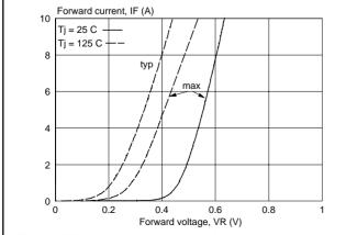
Fig.3. Typical and maximum forward characteristic per diode  $I_F = f(V_F)$ ; parameter  $T_i$
