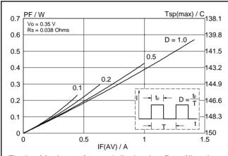
Fig.2. Maximum forward dissipation  $P_F = f(I_{F(AV)})$  per diode; square current waveform where  $I_{F(AV)} = I_{F(RMS)} x \sqrt{D}$ .
