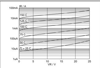
Fig.4. Typical reverse leakage current per diode;  $I_R = f(V_R)$ ; parameter  $T_i$
