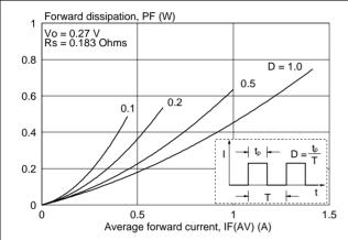
Fig.2. Maximum forward dissipation  $P_F = f(I_{F(AV)})$  per diode; square current waveform where  $I_{F(AV)} = I_{F(RMS)} \times \sqrt{D}$ .
