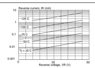
Fig.5. Typical reverse leakage current per diode;  $I_R = f(V_R)$ ; parameter  $T_j$
