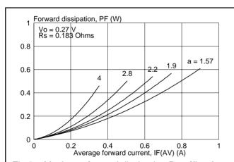
Fig.3. Maximum forward dissipation  $P_F = f(I_{F(AV)})$  per diode; sinusoidal current waveform where a = f form factor  $= I_{F(RMS)} / I_{F(AV)}$ .
