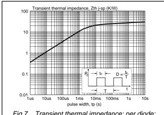
Fig.7. Transient thermal impedance; per diode;  $Z_{th j ext{-}sp} = f(t_p)$ .
