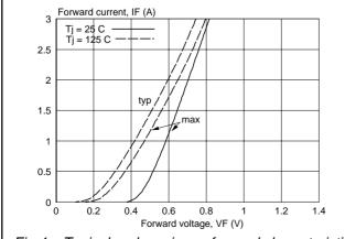
Fig.4. Typical and maximum forward characteristic  $I_F = f(V_F)$ ; parameter  $T_i$
