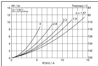
Fig.2. Maximum forward dissipation  $P_F = f(I_{F(AV)})$  per diode; sinusoidal current waveform where a = f form factor  $= I_{F(RMS)} / I_{F(AV)}$ .
