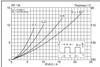
Fig.1. Maximum forward dissipation  $P_F = f(I_{F(AV)})$  per diode; square current waveform where  $I_{F(AV)} = I_{F(RMS)} x \sqrt{D}$ .
