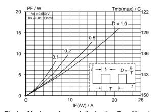
Fig.1. Maximum forward dissipation  $P_F = f(I_{F(AV)})$  per diode; square current waveform where  $I_{F(AV)} = I_{F(RMS)} x \sqrt{D}$ .
