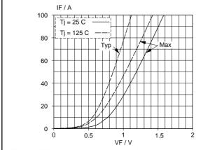
Fig.3. Typical and maximum forward characteristic per diode;  $I_F = f(V_F)$ ; parameter  $T_i$
