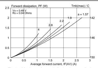
Fig.2. Maximum forward dissipation per diode  $P_F = f(I_{F(AV)})$ ; sinusoidal current waveform where a = f(AV).
