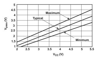
Figure 3. V<sub>pass</sub> Voltage vs V<sub>CC</sub>
