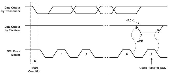
Figure 7. Acknowledgment on the I<sup>2</sup>C Bus
