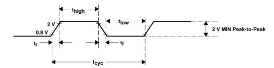
Figure 8–2. PCLK Timing Waveform
