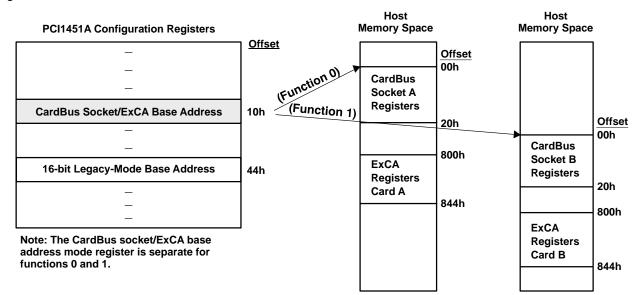
Figure 6–1. Accessing CardBus Socket Registers Through PCI Memory
