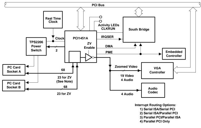
NOTE: The PC Card interface is 68 pins for CardBus and 16-bit PC Cards. In ZV mode, 23 pins are used for routing the ZV signals to the VGA controller and audio subsystem.
