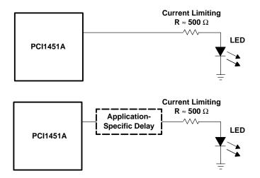
Figure 3–14. Two Sample LED Circuits
