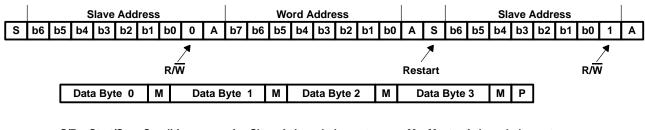
S/P – Start/Stop Condition A – Slave Acknowledgment M – Master Acknowledgment
