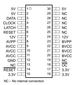
Figure 3–8. TPS2206 Terminal Assignments
