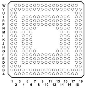
Figure 2–1. PCI1451A GJG Terminal Diagram
