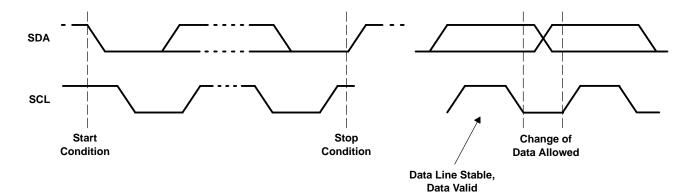
Figure 3–5. Serial EEPROM Start/Stop Conditions and Bit Transfers
