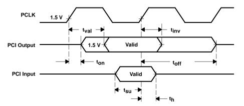
Figure 8-4. Shared Signals Timing Waveforms
