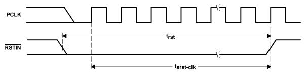
Figure 8–3. RSTIN Timing Waveforms
