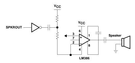
Figure 3–13. Simplified Test Schematic
