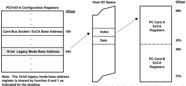
Offset of desired register is placed in the Index register and the data from that location is returned in the data register.
