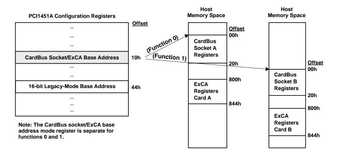
Offsets are from the CardBus socket/ExCA base address register's base address.
