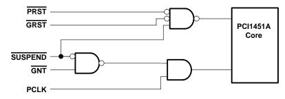
Figure 3–16. SUSPEND Functional Illustration
