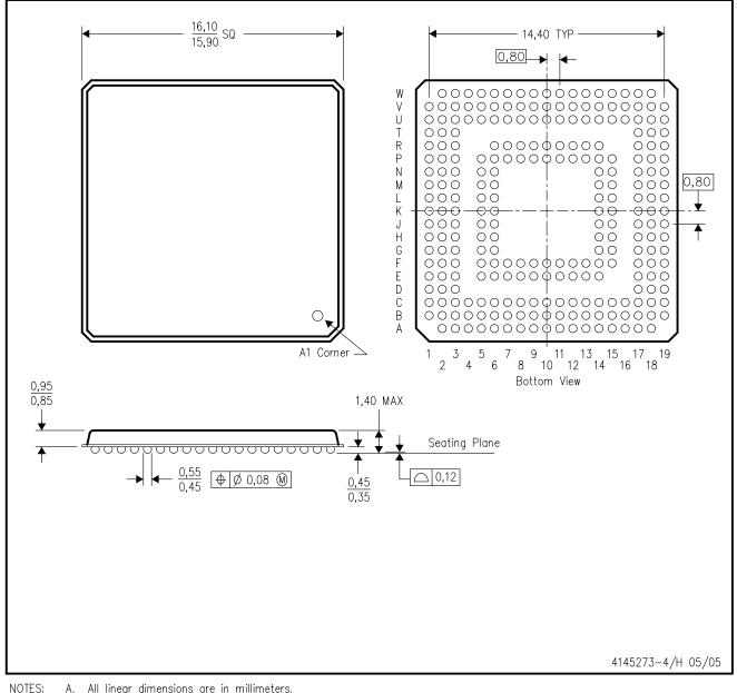
A. All linear dimensions are in millimeters.
