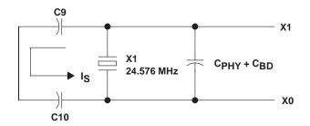
Figure 3–20. Load Capacitance for the PCI7x21/PCI7x11 PHY
