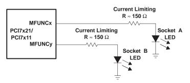
Figure 3-6. Two Sample LED Circuits
