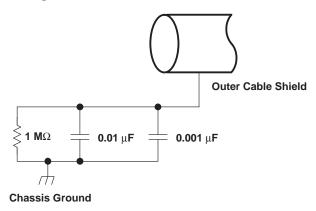
Figure 3–18. Typical Compliant DC Isolated Outer Shield Termination
