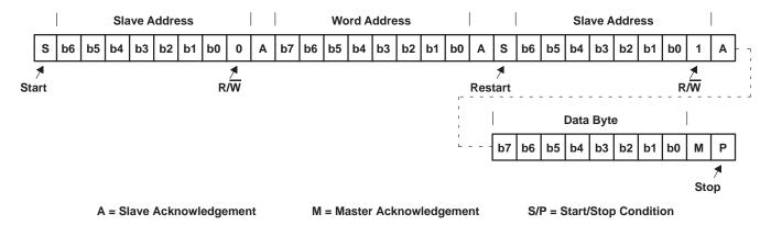
Figure 3-10. Serial-Bus Protocol—Byte Read
