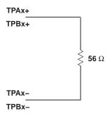
Figure 14-1. Test Load Diagram
