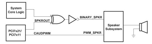
Figure 3–5. SPKROUT Connection to Speaker Driver
