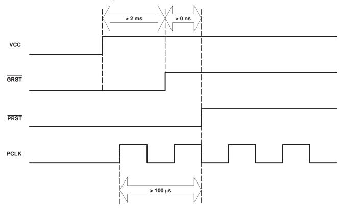
Figure 3-3. PCI Reset Requirement
