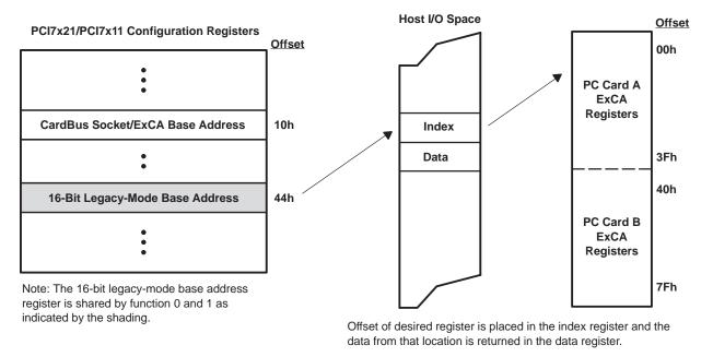
Figure 5-1. ExCA Register Access Through I/O
