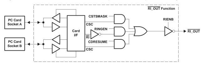
Figure 3–15. RI OUT Functional Diagram
