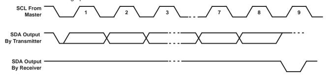
Figure 3-8. Serial-Bus Protocol Acknowledge
