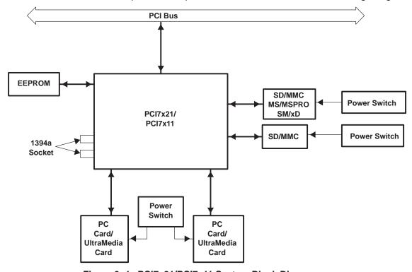
Figure 3-1. PCI7x21/PCI7x11 System Block Diagram
