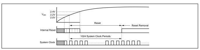
FIGURE 3. Power-On Reset Timing
