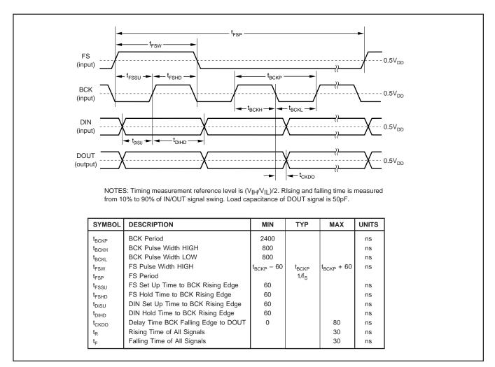
FIGURE 7. Serial Interface Timing for Slave Mode.
