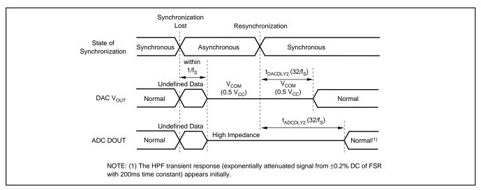
FIGURE 10. Loss of Synchronization Operation and Timing.
