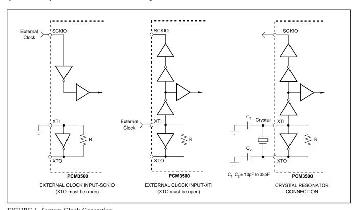
FIGURE 1. System Clock Generation.
