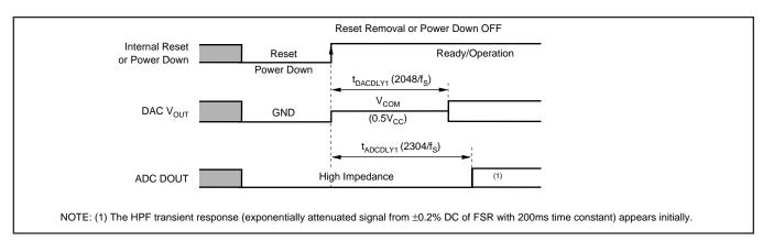
FIGURE 5. DAC and ADC Output for Reset and Power Down.
