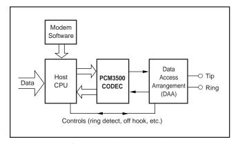
FIGURE 24. Software Modem Block Diagram.
