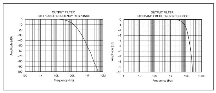
FIGURE 20. DAC Output Amplifier Filter Response.
