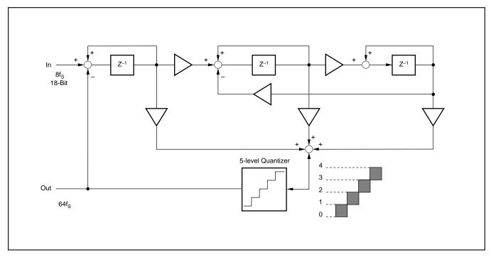
FIGURE 27. 5-Level Delta-Sigma Modulator Block Digram.
