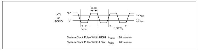
FIGURE 2. External System Clock Timing Requirements.
