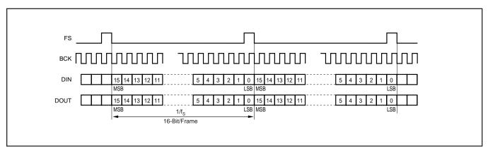
FIGURE 6. Serial Interface Format.
