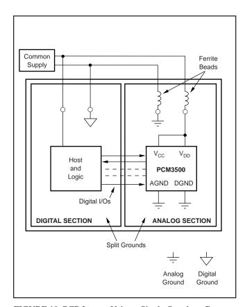
FIGURE 19. PCB Layout Using a Single-Supply or Battery.
