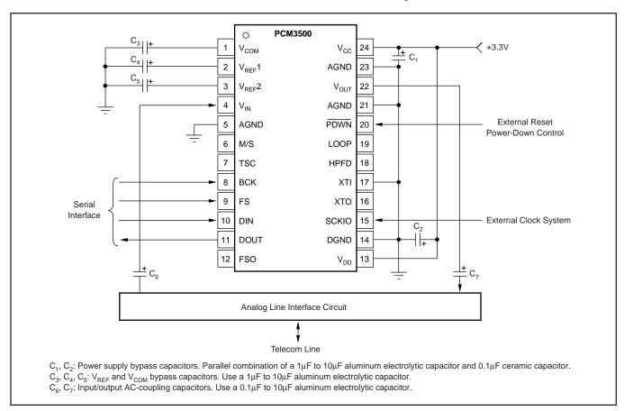
FIGURE 16. Basic Connection Diagram.
