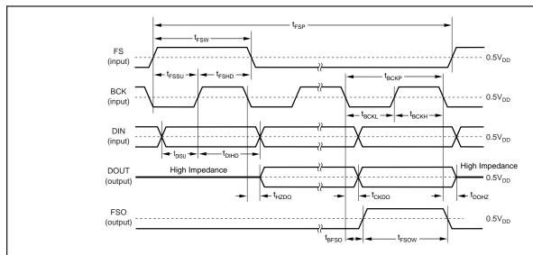
NOTES: Timing measurement reference level is  $(V_{IH}/V_{IL})/2$ . Rising and falling time is measured from 10% to 90% of IN/OUT signal swing. Load capacitance of DOUT, and FSO signal is 50pF.
