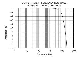
$T_{A}$  = +25°C,  $V_{CC}$  =  $V_{DD}$  = +3.3V,  $f_{S}$  = 8kHz, and  $f_{SIGNAL}$  = 1kHz, unless otherwise specified.
