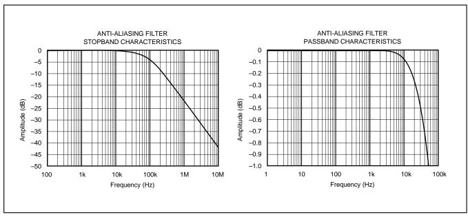
FIGURE 22. Anti-Alias Filter Frequency Response.
