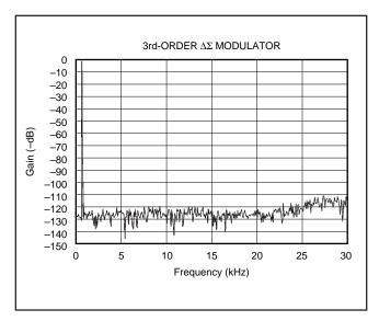
FIGURE 28. Quantization Noise Spectrum.
