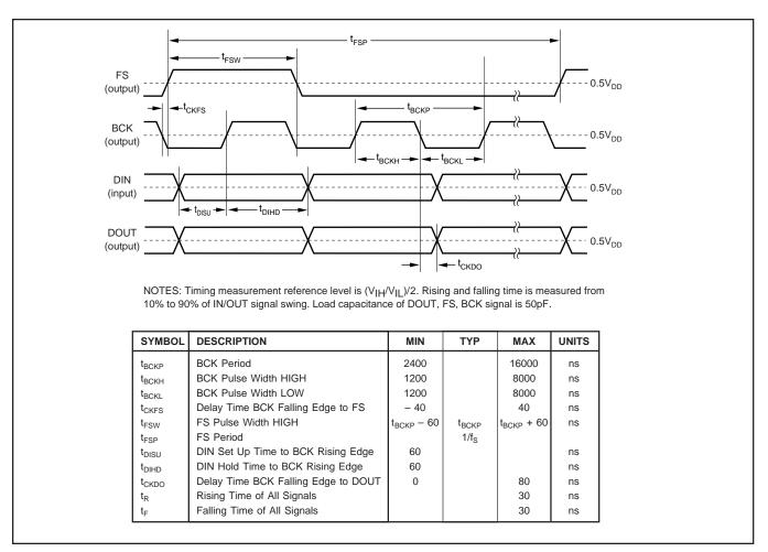
FIGURE 8. Serial Interface Timing for Master Mode.
