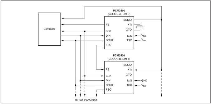
FIGURE 11. Time Slot Mode Connections.
