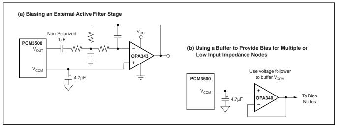
FIGURE 17. Using V<sub>COM</sub> to Bias External Circuitry.
