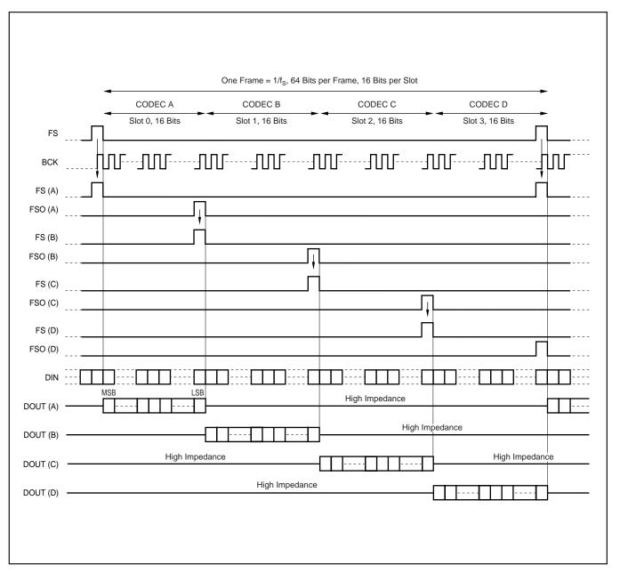
FIGURE 12. Time Slot Mode Operation.
