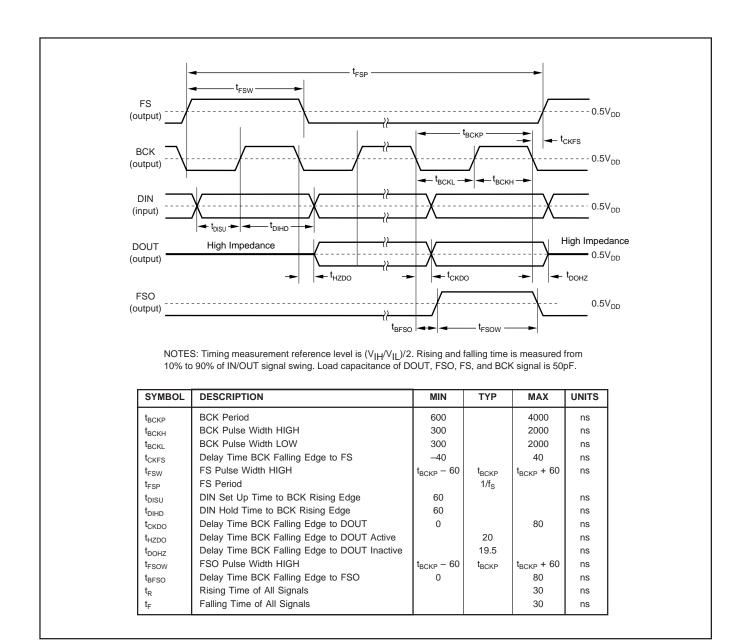
FIGURE 14. Serial Interface Timing for Time Slot Mode Operation (Master Mode).
