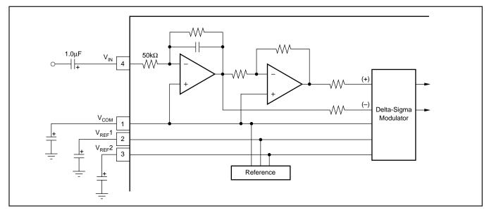
FIGURE 21. On-Chip AFE Circuit for the ADC.
