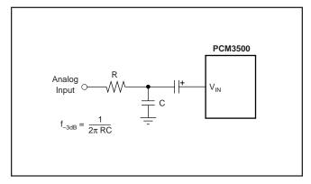
FIGURE 23. Optional External Low-Pass Filter for the ADC.
