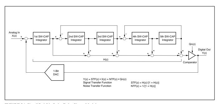
FIGURE 26. Simplified 5th-Order Delta-Sigma Modulator.
