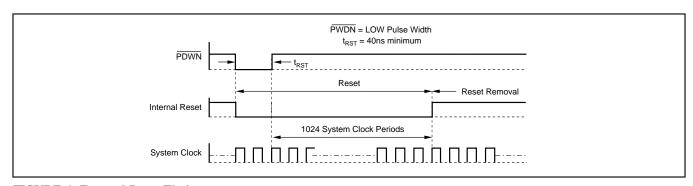
FIGURE 4. External Reset Timing.
