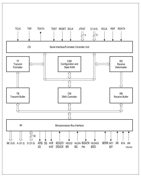
Figure 3 Block Diagram of MUNICH32
