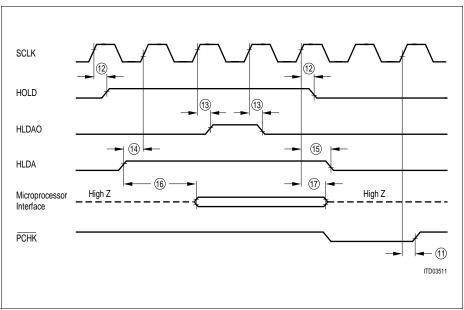
Figure 120 Bus Arbitration Timing Diagram Intel Bus Mode
