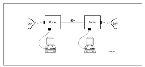
Figure 85 ISDN/LAN Router
