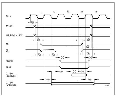
Figure 121 Timing Diagram Motorola Bus Mode
