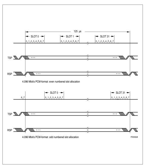
Figure 15 4.096 Mbit/s PCM Frame Timing
