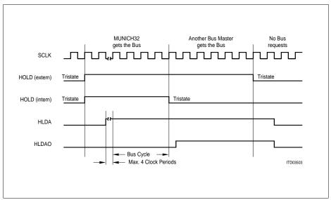
Figure 20 Bus Management for Intel Bus Mode
