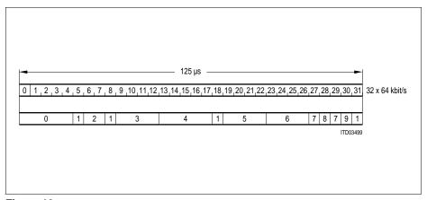
Figure 16 Example: Programmable Channel Allocation for 32 Time Slots
