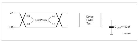
Figure 118 Input/Output Waveform for AC Tests
