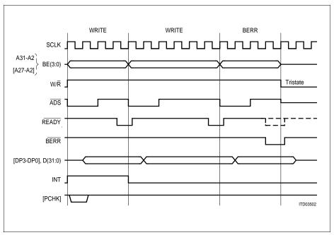
Figure 19 Write Cycle Timing Diagram (Intel mode)
