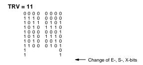
For INV = 1 (channel inversion) all bits are inverted. For Motorola mode the data sections would have to have the form to yield the same output data.
