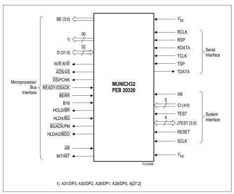
Figure 2 MUNICH32 Logic Symbol
