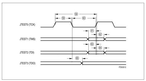
Figure 126 JTAG-Boundary Scan Timing
