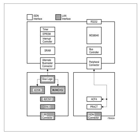
Figure 86 Hardware Block Diagram
