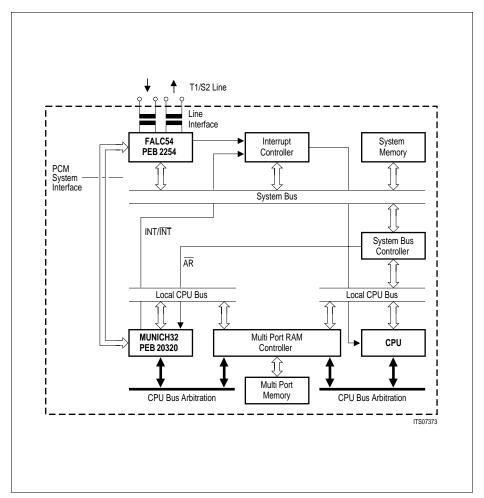
Figure 11 MUNICH32 in a System using Multiport Memory
