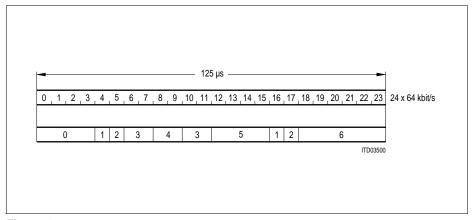
Figure 17 Example: Programmable Channel Allocation for 24 Time Slots
