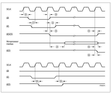
Figure 122 Bus Arbitration Timing Motorola Bus Mode
