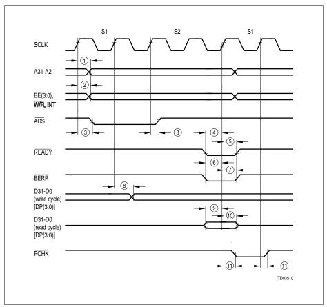
Figure 119 Timing Diagram Intel Bus Mode
