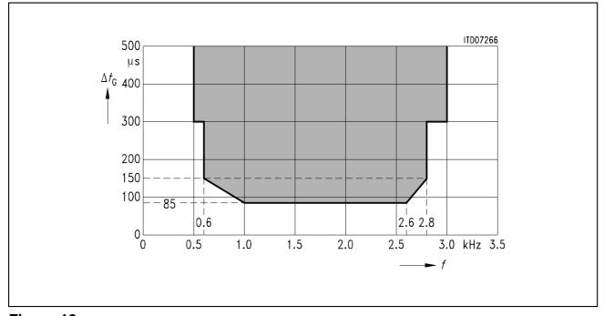
Figure 18 Group Delay Distortion Receive: Input Signal Level 0 dBm0<sup>1)</sup>
