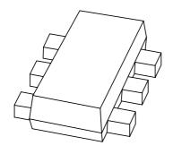
PESD3V3L5UV; PESD5V0L5UV Low capacitance 5-fold ESD protection diode arrays in SOT666 package
