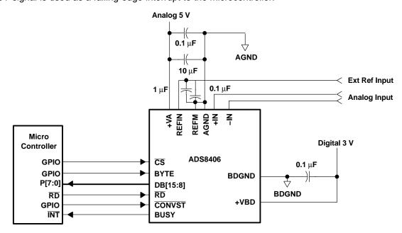
Figure 31. ADS8406 Application Circuitry (using external reference)
