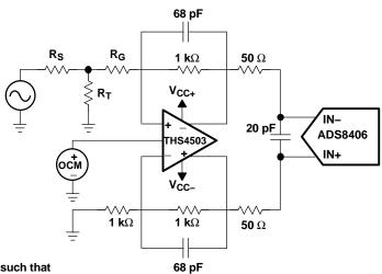
$R_{G},\,R_{S},$  and  $R_{T}$  should be chosen such that  $R_{G+}\,R_{S}\mid\mid R_{T}$  = 1 k  $\Omega$  V  $_{OCM}$  = 2 V, +V  $_{CC}$  = 7 V, and -V  $_{CC}$  = -7 V
