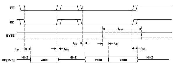
Figure 5. Detailed Timing for Read Cycles
