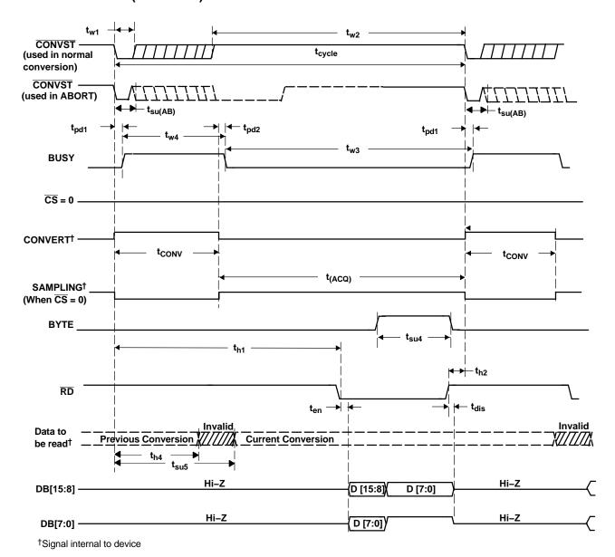
Figure 3. Timing for Conversion and Acquisition Cycles With CS Tied to BDGND, RD Toggling
