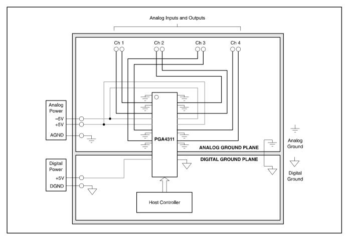
Figure 6. Typical PCB Layout Floor Plan.
