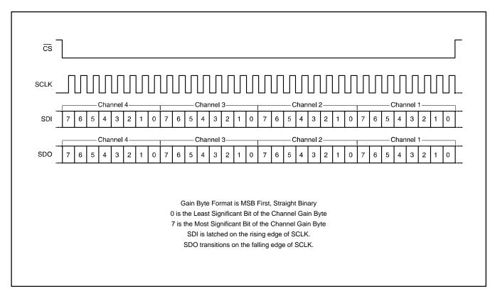
Figure 2. Serial Interface Protocol.
