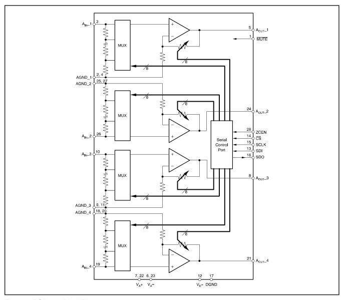
Figure 1. PGA4311 Block Diagram.
