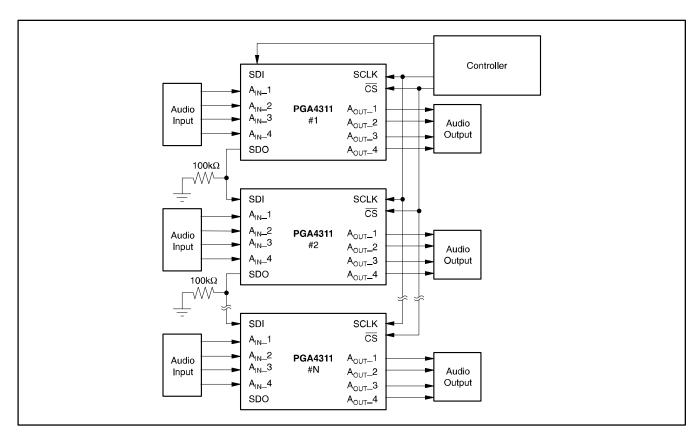
Figure 4. Daisy-Chaining Multiple PGA4311 Devices.
