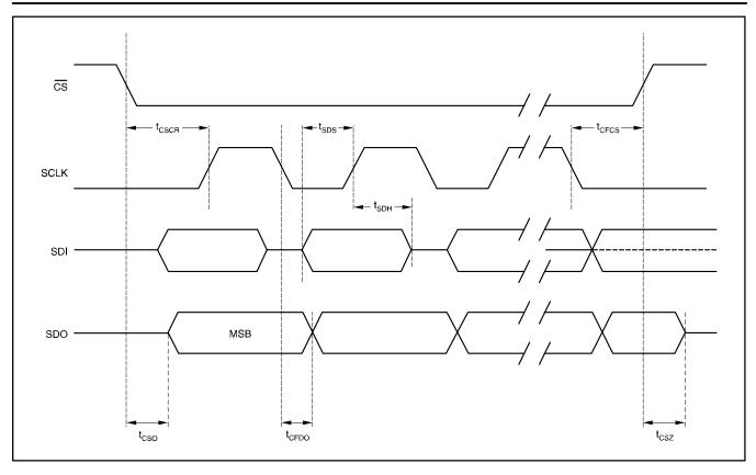
Figure 3. Serial Interface Timing Requirements.
