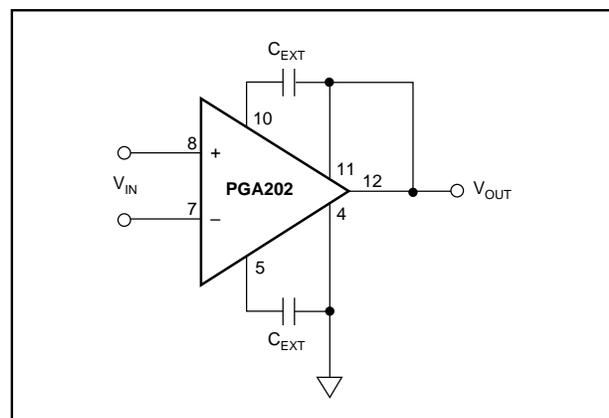
FIGURE 5. Output Filtering.
