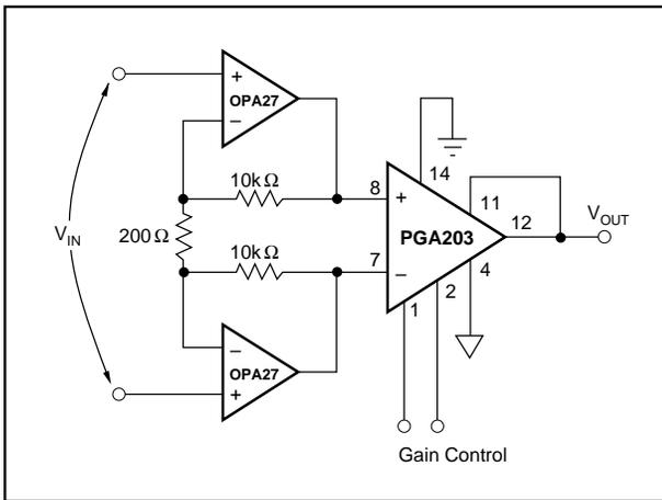
FIGURE 10. Low Noise Differential Amplifier with Gains of 100, 200, 400, 800.
