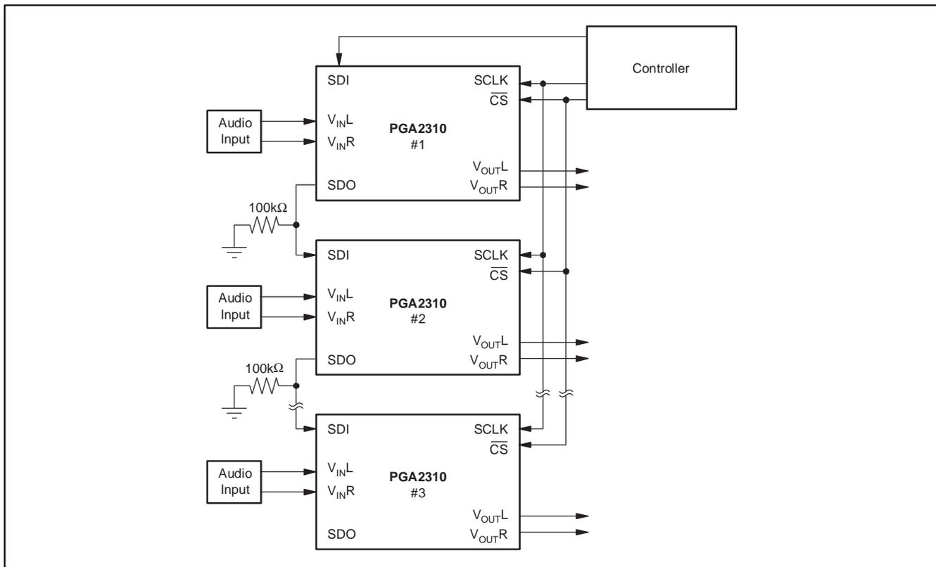
**Figure 4. Daisy-Chaining Multiple PGA2310 Devices**
