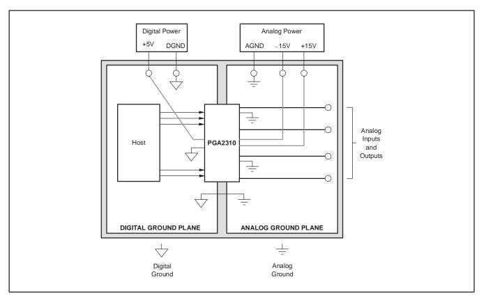
Figure 6. Typical PCB Layout Floor Plan
