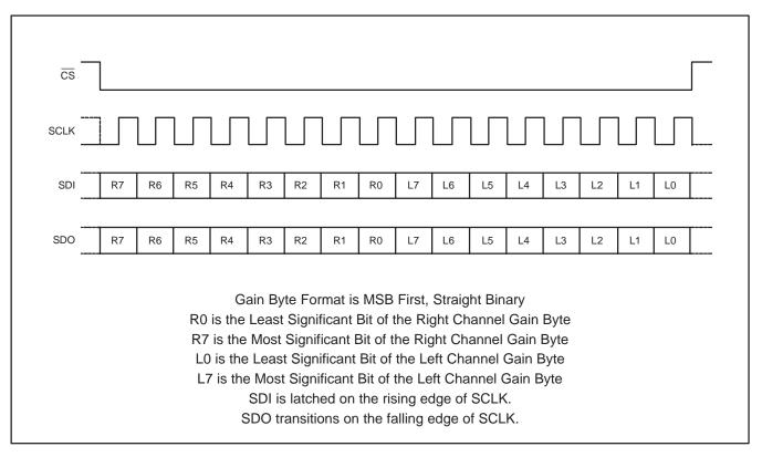
Figure 2. Serial Interface Protocol
