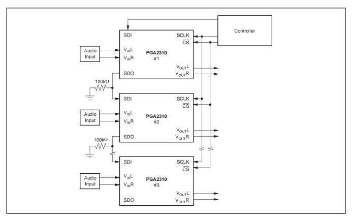
Figure 4. Daisy-Chaining Multiple PGA2310 Devices
