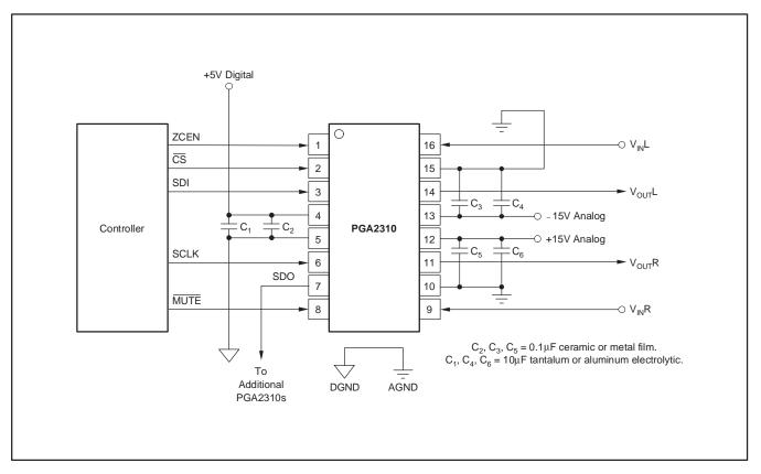
Figure 5. Recommended Connection Diagram
