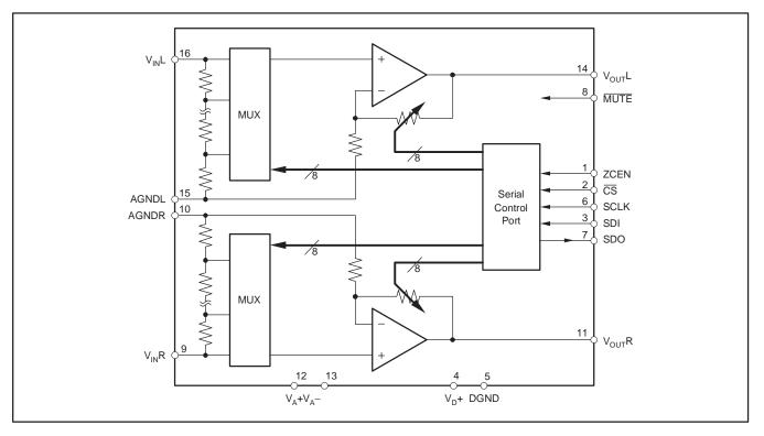
Figure 1. PGA2310 Block Diagram
