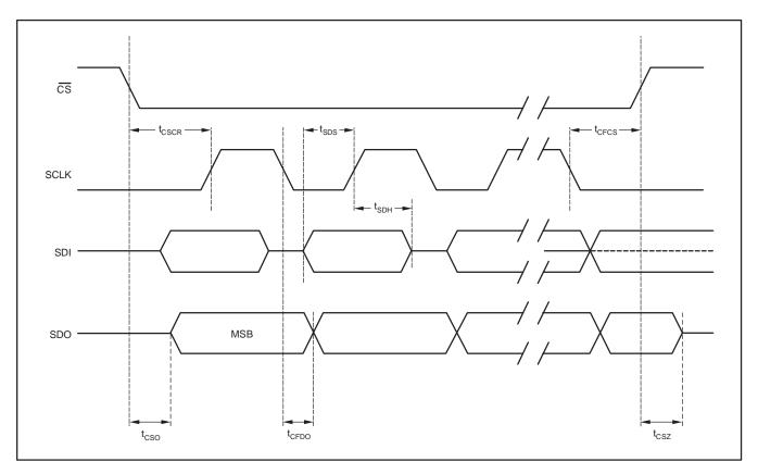
Figure 3. Serial Interface Timing Requirements
