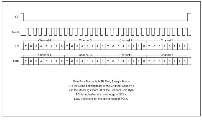
Figure 2. Serial Interface Protocol.
