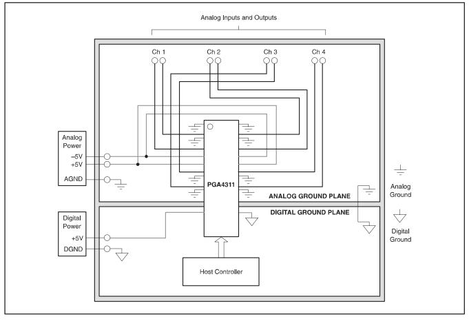
Figure 6. Typical PCB Layout Floor Plan.
