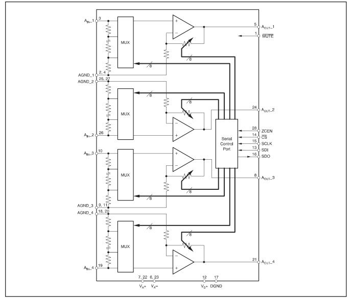
Figure 1. PGA4311 Block Diagram.
