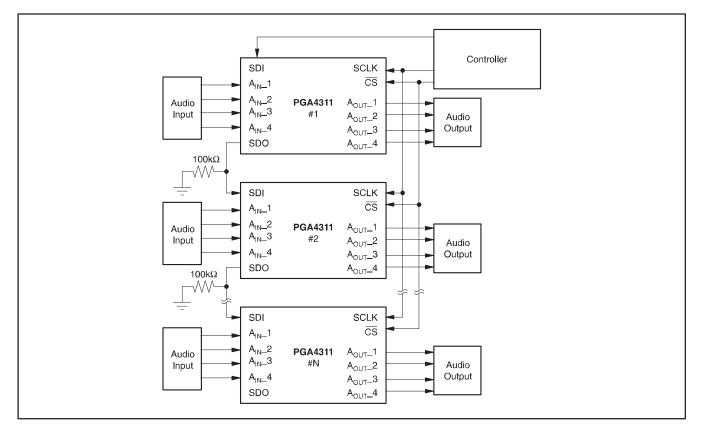
Figure 4. Daisy-Chaining Multiple PGA4311 Devices.
