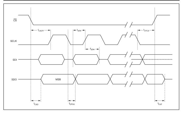
Figure 3. Serial Interface Timing Requirements.
