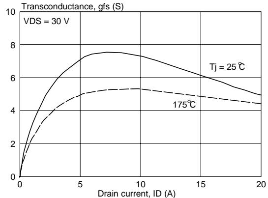
Fig.8. Typical transconductance,  $T_j = 25^\circ\text{C}$ .
