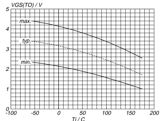
Fig.10. Gate threshold voltage.
