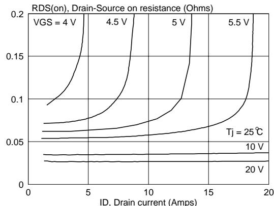
Fig.6. Typical on-state resistance,  $T_j = 25^\circ\text{C}$ .
