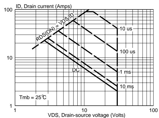
Fig.3. Safe operating area.  $T_{mb} = 25^\circ\text{C}$
