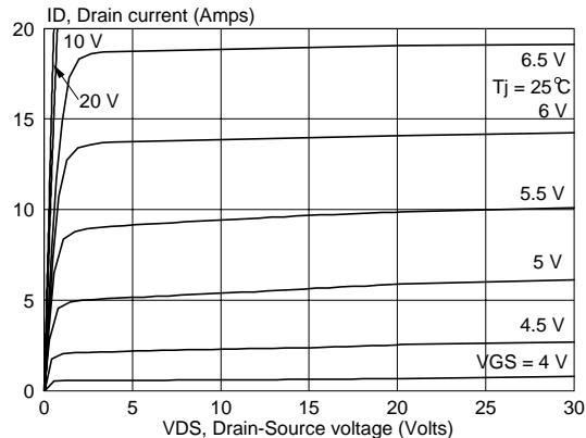
Fig.5. Typical output characteristics,  $T_j = 25^\circ\text{C}$ .
