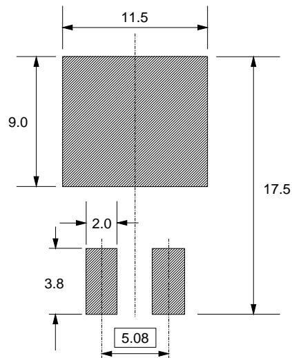
Fig.18. SOT404 : soldering pattern for surface mounting.
