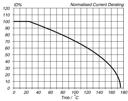
Fig.2. Normalised continuous drain current.
