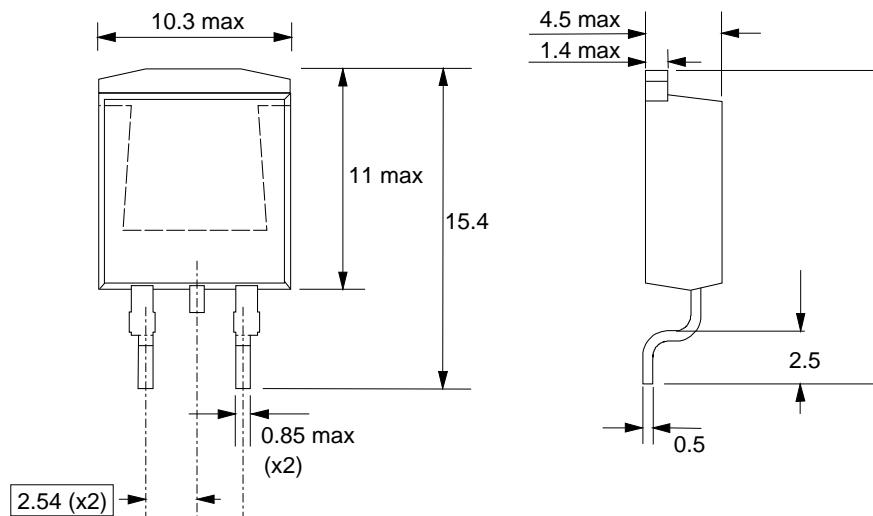
Fig.17. SOT404 : centre pin connected to mounting base.
