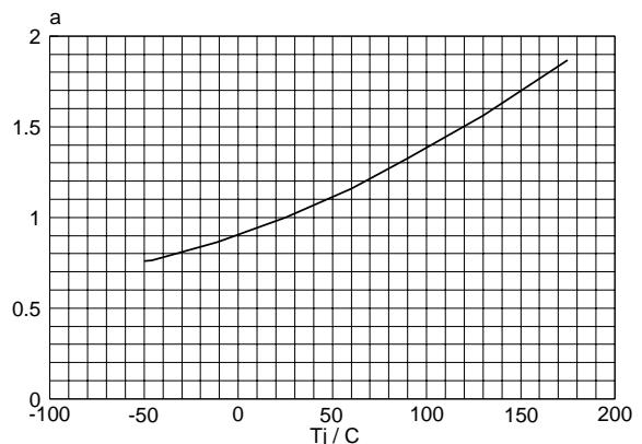
Fig.9. Normalised drain-source on-state resistance.
