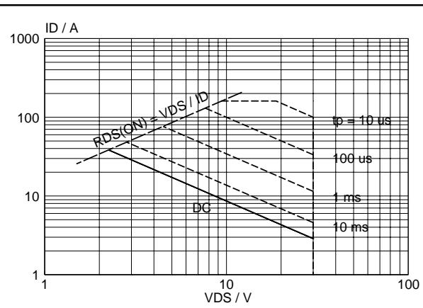
*Fig.3. Safe operating area,  $T_{mb} = 25 \text{ } ^{\circ}\text{C}$*
