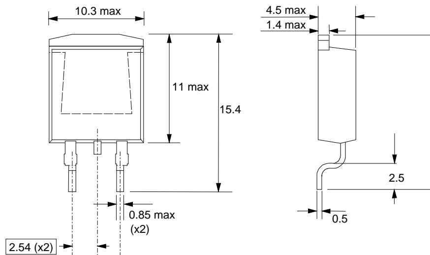
Fig.18. SOT404 : centre pin connected to mounting base.
