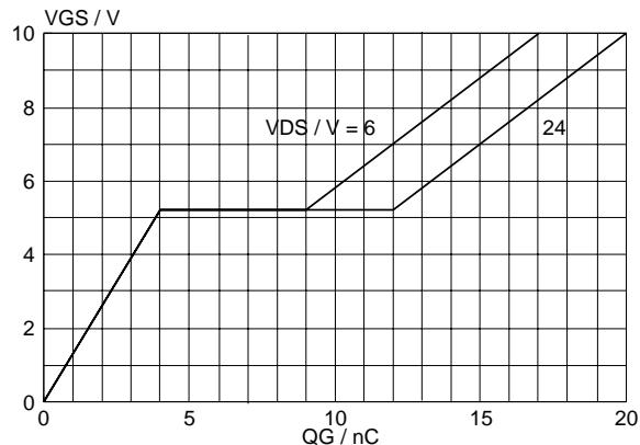
Fig.13. Typical turn-on gate-charge characteristics.
