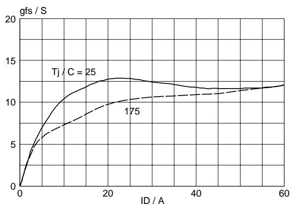
Fig. 8. Typical transconductance,  $T_j = 25$  °C.
