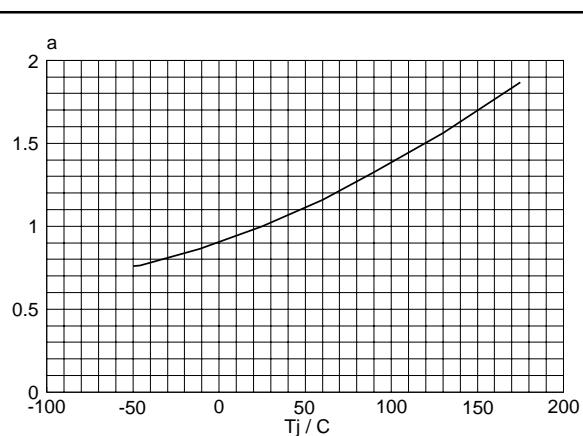
Fig. 9. Normalised drain-source on-state resistance.
