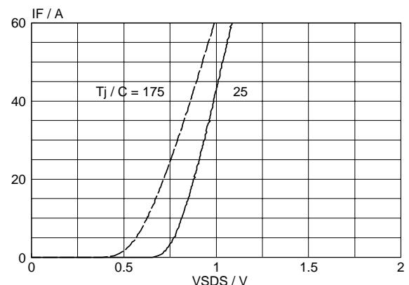
Fig.14. Typical reverse diode current.
