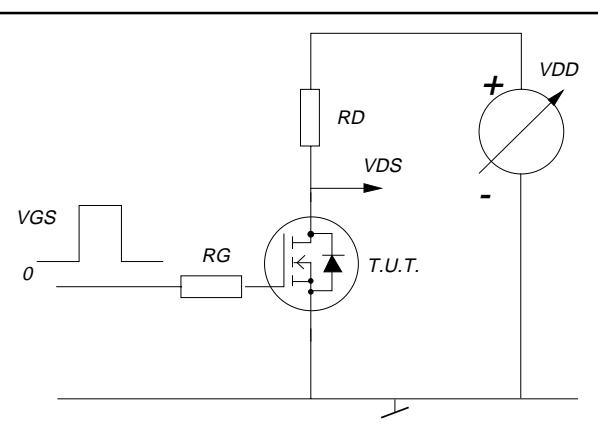
Fig.17. Switching test circuit.
