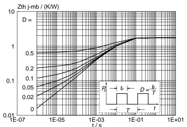
*Fig.4. Transient thermal impedance.*
