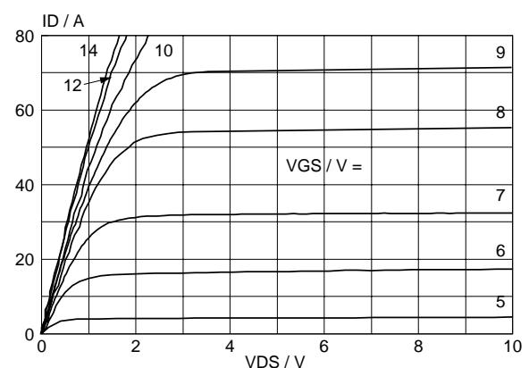
*Fig.5. Typical output characteristics,  $T_j = 25 \text{ } ^{\circ}\text{C}$ .*
