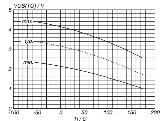
Fig. 10. Gate threshold voltage.
