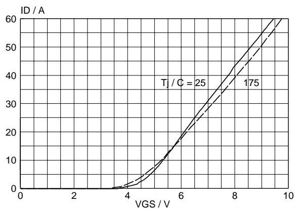
Fig. 7. Typical transfer characteristics.
