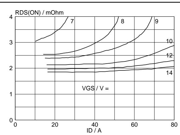
*Fig.6. Typical on-state resistance,  $T_j = 25 \text{ } ^{\circ}\text{C}$ .*
