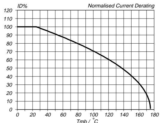
*Fig.2. Normalised continuous drain current.*
