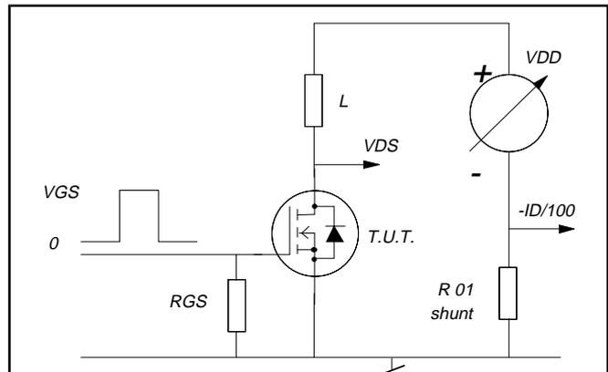
Fig.16. Avalanche energy test circuit.
