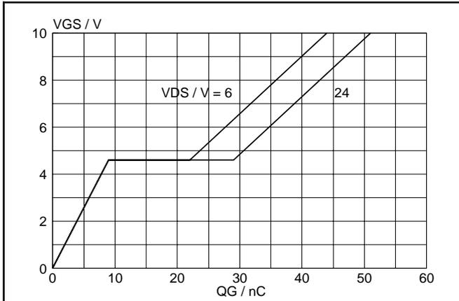
Fig.13. Typical turn-on gate-charge characteristics.
