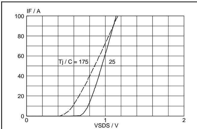
Fig.14. Typical reverse diode current.
