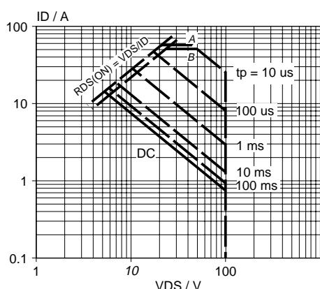
Fig.3. Safe operating area.  $T_{mb} = 25 \text{ } ^\circ C$
