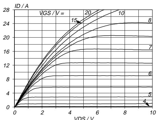
Fig.5. Typical output characteristics,  $T_j = 25 \text{ } ^\circ C$ .
