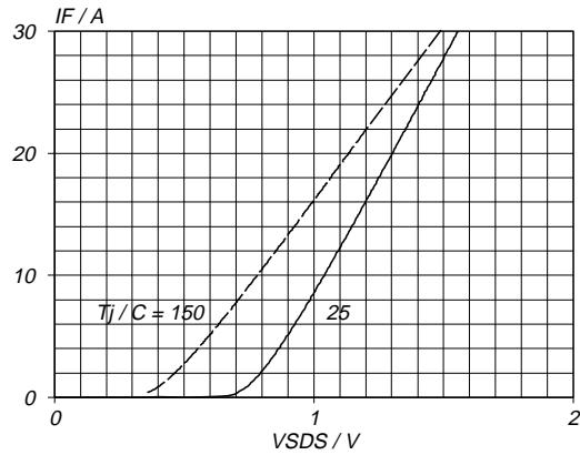
Fig.14. Typical reverse diode current.
