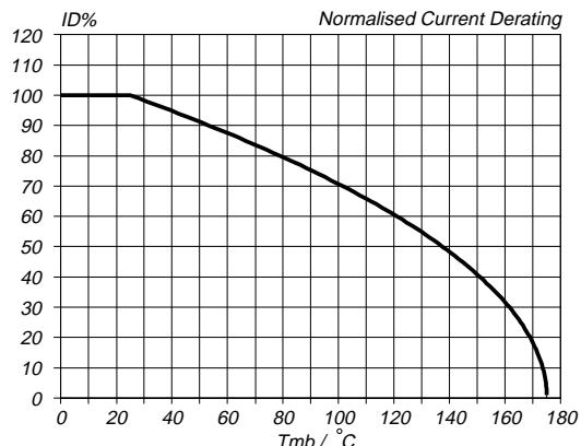
Fig.2. Normalised continuous drain current.
