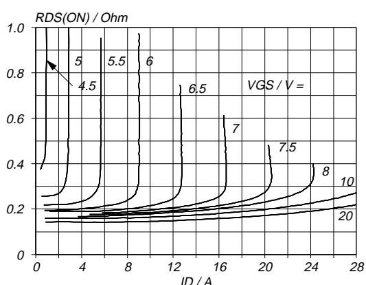
Fig.6. Typical on-state resistance,  $T_j = 25 \text{ } ^\circ C$ .
