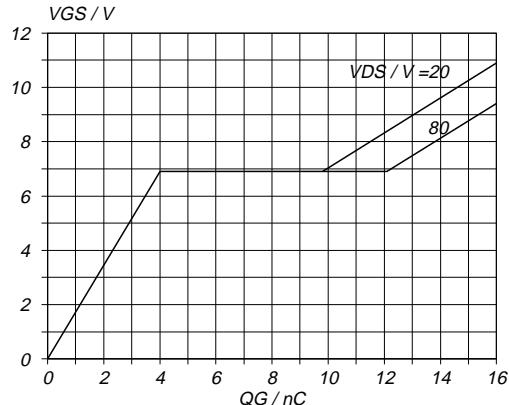
Fig.13. Typical turn-on gate-charge characteristics.
