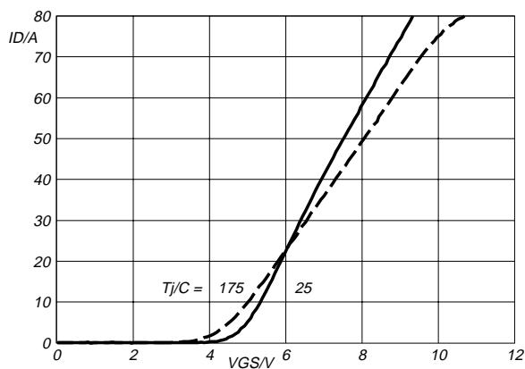
Fig. 7. Typical transfer characteristics.
