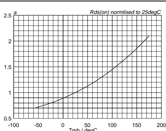
Fig. 9. Normalised drain-source on-state resistance.
