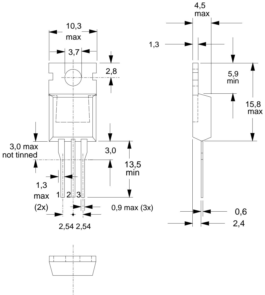
Fig.18. SOT78 (TO220AB); pin 2 connected to mounting base.
