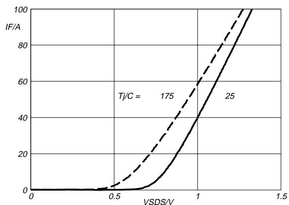
Fig.14. Typical reverse diode current.
