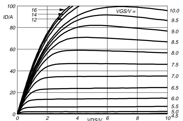
Fig.5. Typical output characteristics,  $T_j = 25$  °C.
