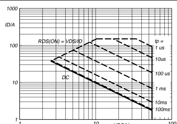
Fig.3. Safe operating area.  $T_{mb} = 25$  °C
