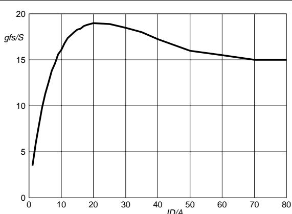
Fig. 8. Typical transconductance,  $T_j = 25$  °C.
