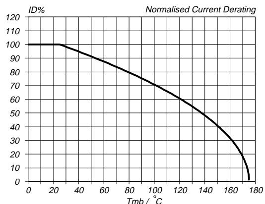
Fig.2. Normalised continuous drain current.
