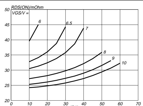
Fig.6. Typical on-state resistance,  $T_j = 25$  °C.
