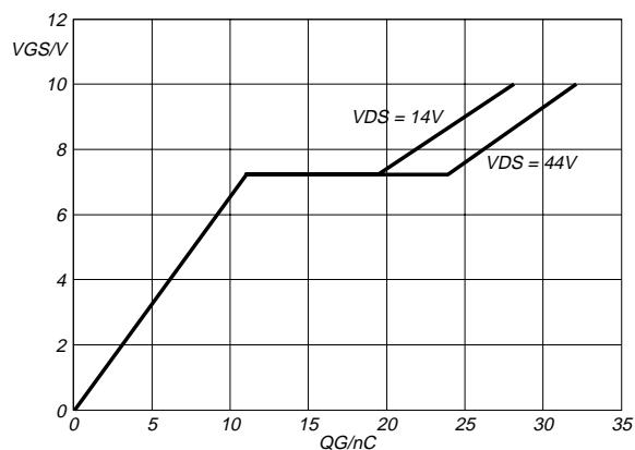
Fig.13. Typical turn-on gate-charge characteristics.
