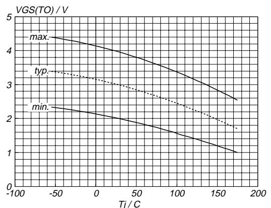
Fig. 10. Gate threshold voltage.
