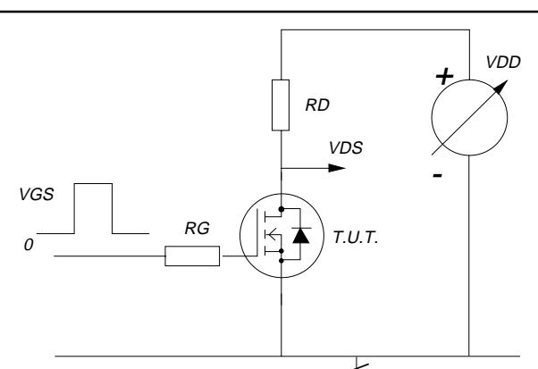
Fig.17. Switching test circuit.
