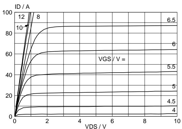
*Fig. 5. Typical output characteristics,  $T_j = 25^\circ C$ .*
