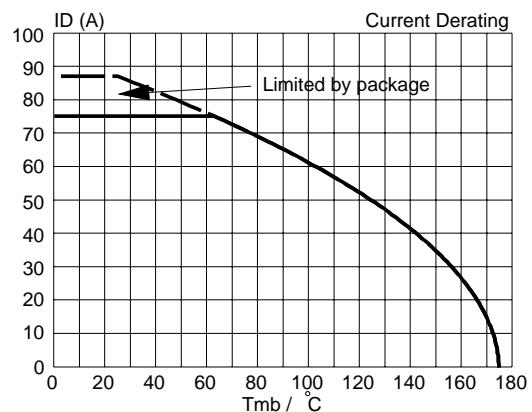
*Fig. 2. Normalised continuous drain current.*
