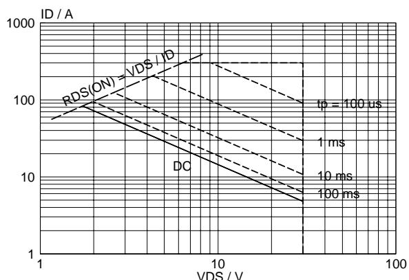
*Fig. 3. Safe operating area.  $T_{mb} = 25^\circ C$*
