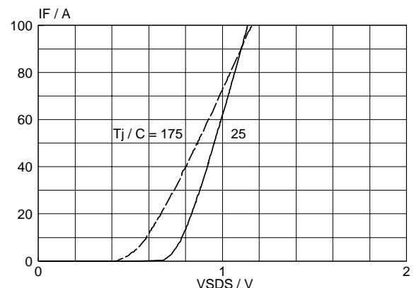
Fig.14. Typical reverse diode current.
