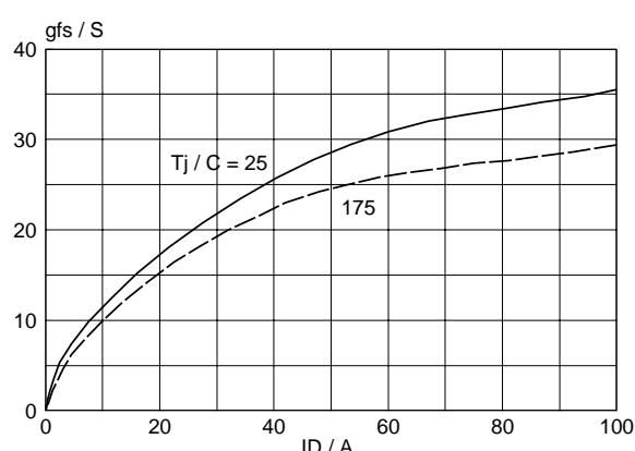
Fig.8. Typical transconductance,  $T_j = 25$  °C.
