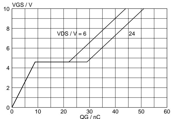
Fig.13. Typical turn-on gate-charge characteristics.
