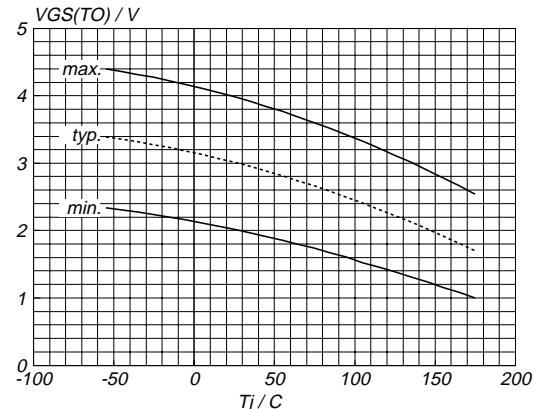
Fig.10. Gate threshold voltage.
