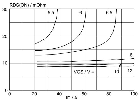
*Fig. 6. Typical on-state resistance,  $T_j = 25^\circ C$ .*
