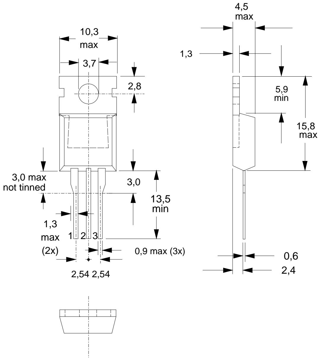
*Fig.18. TO220AB; pin 2 connected to mounting base.*
