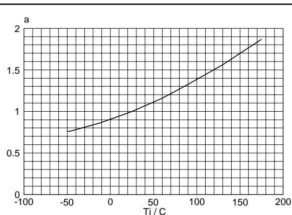
Fig.9. Normalised drain-source on-state resistance.
