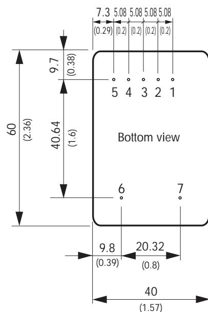
Pin diameter  $\varnothing 0.8 \pm 0.05$  (0.03)  $\pm 0.002$
