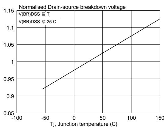
Fig.15. Normalised drain-source breakdown voltage;
