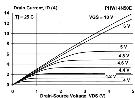
Fig.5. Typical output characteristics.
