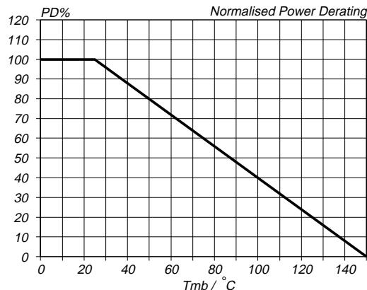
Fig.1. Normalised power dissipation.
