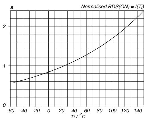
Fig.9. Normalised drain-source on-state resistance.
