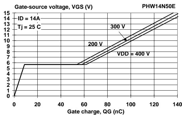
Fig.13. Typical turn-on gate-charge characteristics.
