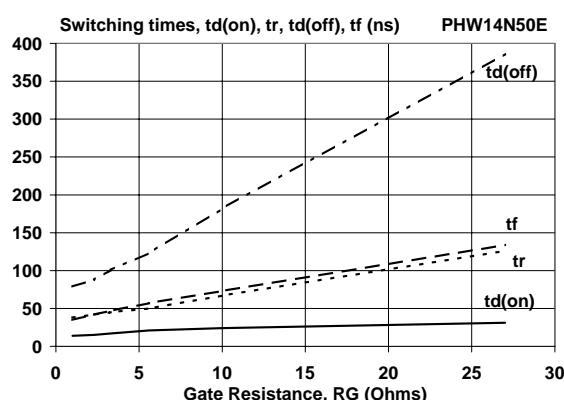
Fig.14. Typical switching times;  $t_{d(on)}$ ,  $t_r$ ,  $t_{d(off)}$ ,  $t_f = f(R_G)$
