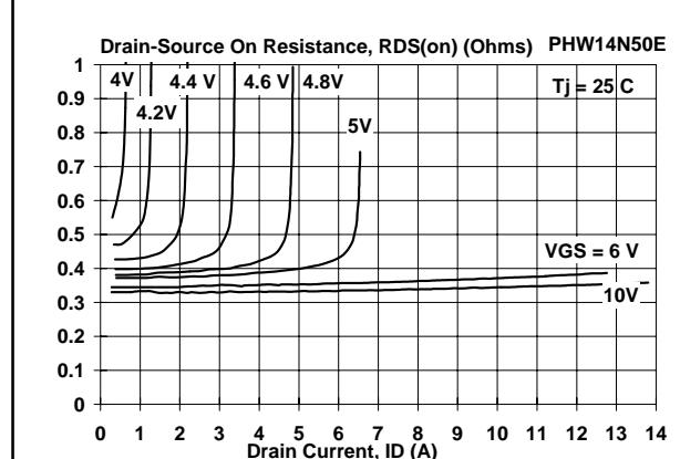
Fig.6. Typical on-state resistance.
