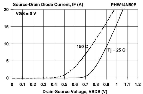
Fig.16. Source-Drain diode characteristic.
