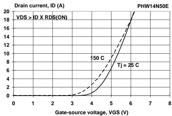
Fig.7. Typical transfer characteristics.
