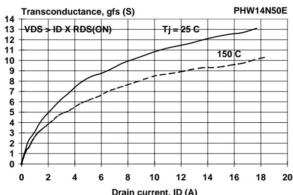
Fig.8. Typical transconductance.
