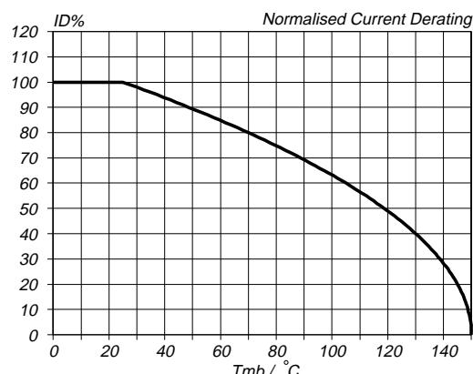
Fig.2. Normalised continuous drain current.
