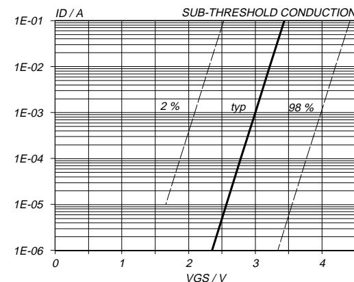
Fig.11. Sub-threshold drain current.
