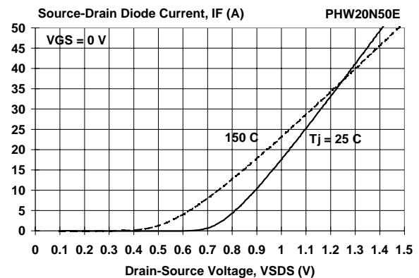
Fig.16. Source-Drain diode characteristic.
