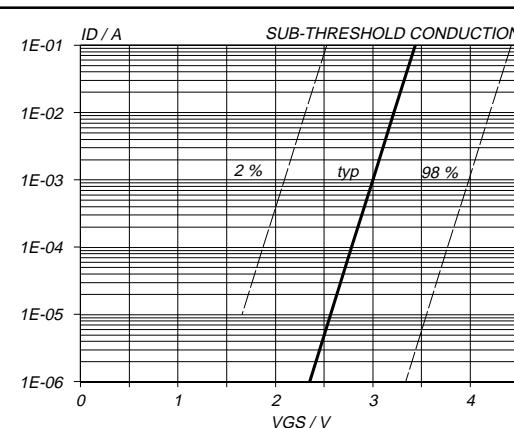
Fig.11. Sub-threshold drain current.
