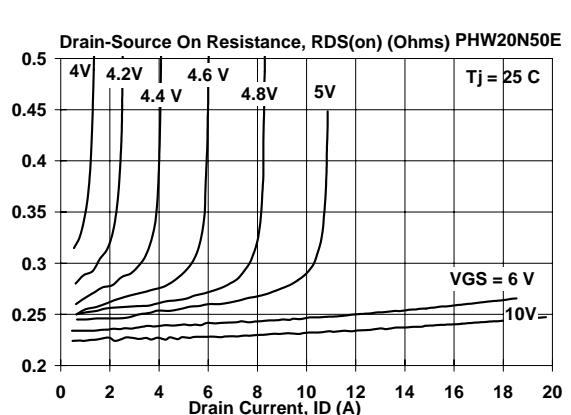
Fig.6. Typical on-state resistance.
