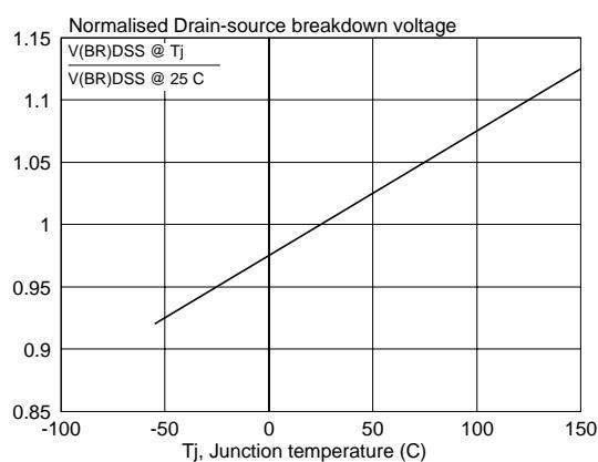
Fig.15. Normalised drain-source breakdown voltage;
