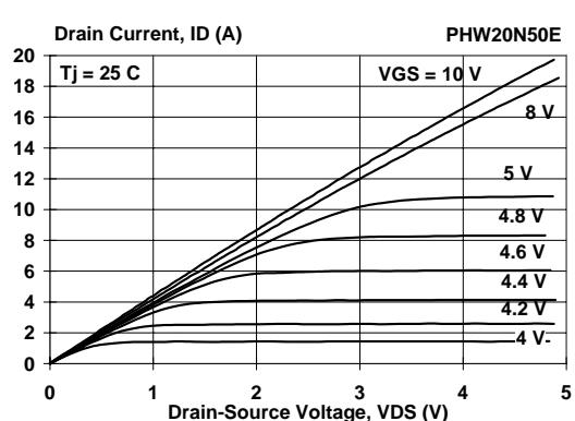
Fig.5. Typical output characteristics.
