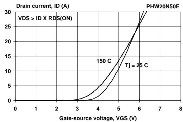
Fig.7. Typical transfer characteristics.
