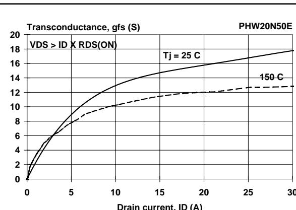
Fig.8. Typical transconductance.
