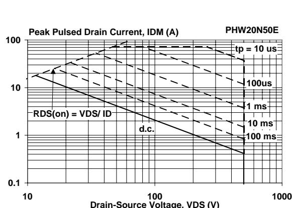
Fig.3. Safe operating area.  $T_{mb} = 25\ ^\circ C$
