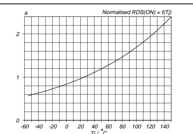
Fig.9. Normalised drain-source on-state resistance.
