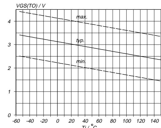
Fig.10. Gate threshold voltage.
