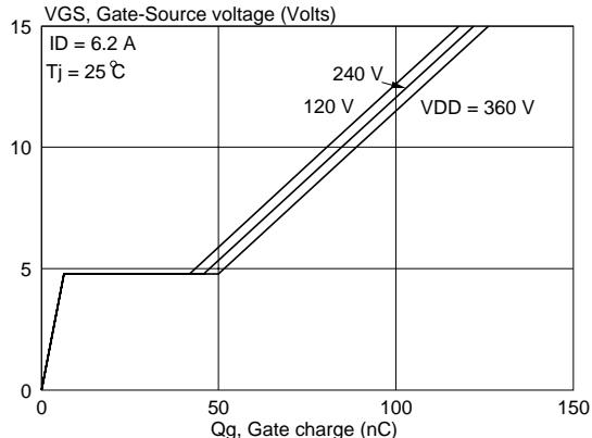
Fig. 13. Typical turn-on gate-charge characteristics.
