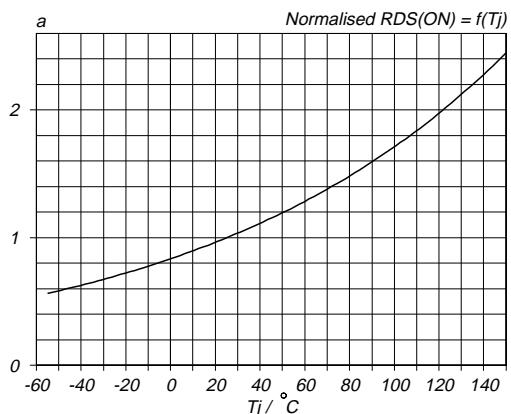
Fig.9. Normalised drain-source on-state resistance.
