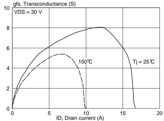
Fig.8. Typical transconductance.
