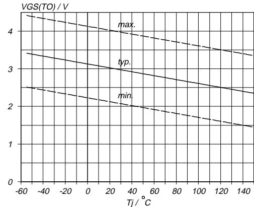
Fig.10. Gate threshold voltage.
