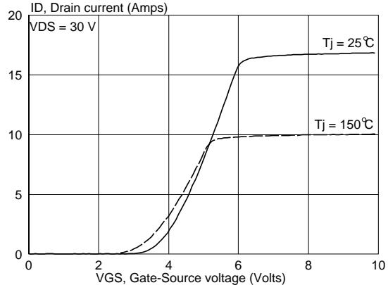
Fig.7. Typical transfer characteristics.
