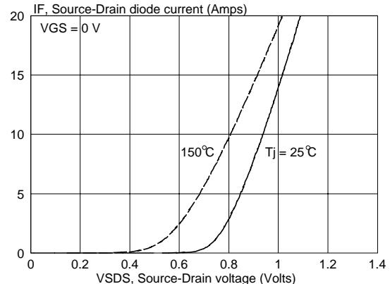
Fig. 16. Source-Drain diode characteristic.
