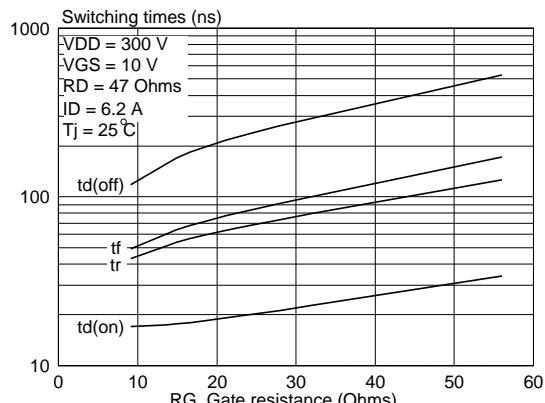
Fig. 14. Typical switching times.
