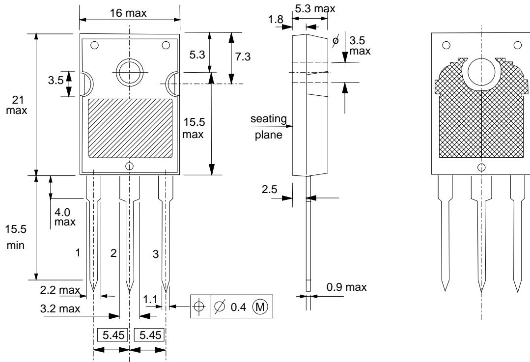
Fig.19. SOT429 (TO247); pin 2 connected to mounting base.
