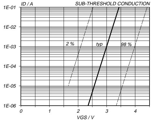
Fig.11. Sub-threshold drain current.
