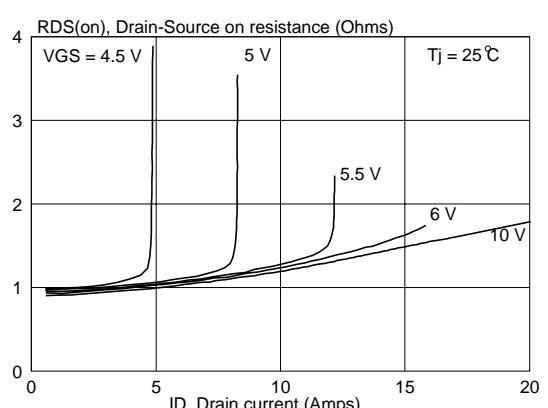
Fig.6. Typical on-state resistance.
