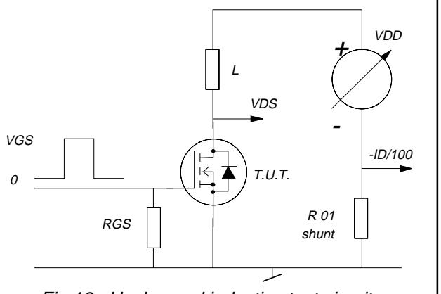
Fig. 18. Unclamped inductive test circuit.
