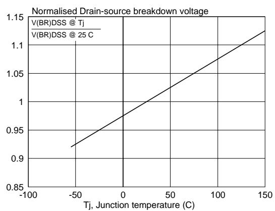
Fig. 15. Normalised drain-source breakdown voltage.
