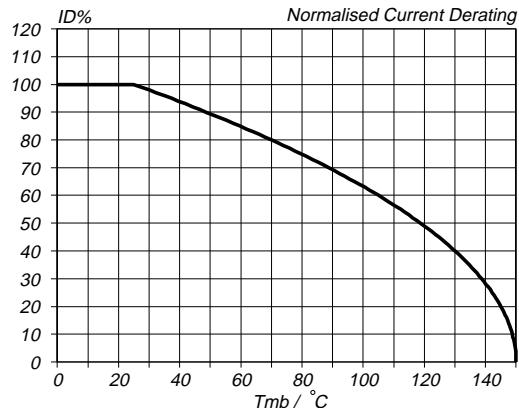
Fig.2. Normalised continuous drain current.
