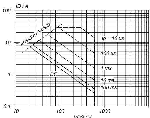
Fig.3. Safe operating area.  $T_{mb} = 25^\circ C$
