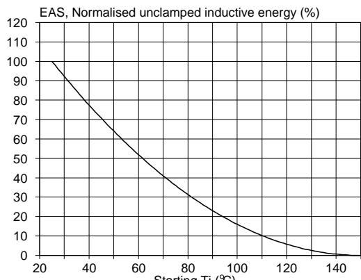
Fig. 17. Normalised unclamped inductive energy.
