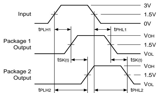
$$t_{sk(t)} = |t_{PLH2} \cdot t_{PLH1}| \text{ or } |t_{PHL2} \cdot t_{PHL1}|$$
