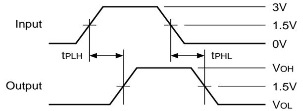
$$t_{sk(p)} = |t_{PHL} \cdot t_{PLH}|$$
