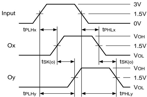
$$t_{sk(o)} = |t_{PLHy} \cdot t_{PLHx}| \text{ or } |t_{PHLy} \cdot t_{PHLx}|$$
